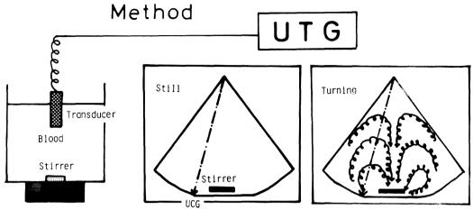
Fig. 2. Experimental schema UCG=M-mode echograms UTG=Ultrasonic tomography
