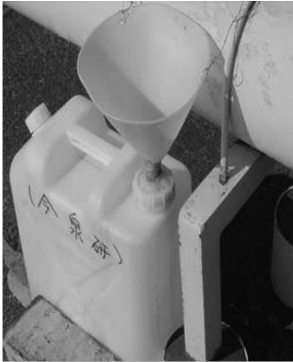
Fig.2.2 The plastic sampler used for collection of monthly precipitation.
