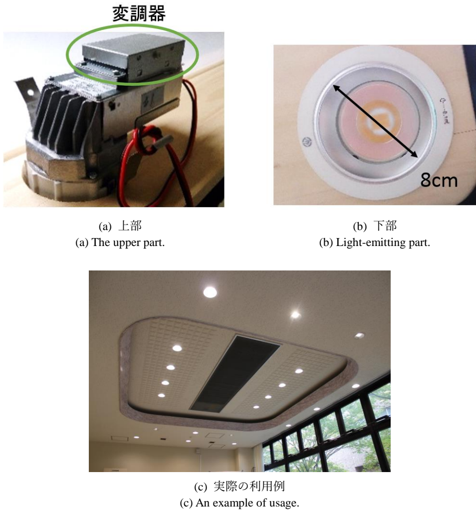
図2 情報送信型 LED 照明 (NNNH73072K) Figure 2 VLC LED light.
