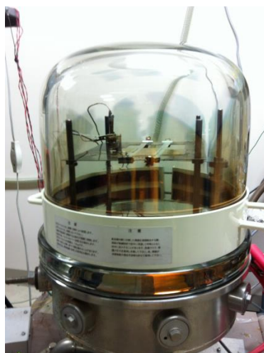
Figure 3.4 The silver electrode deposited by the vacuum evaporation method on the spiro-OMeTAD layer.
