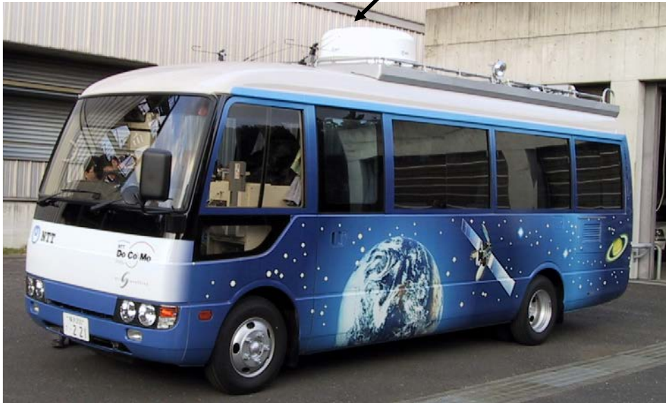
Figure 3-9 Experimented vehicle housing tracking antenna.
