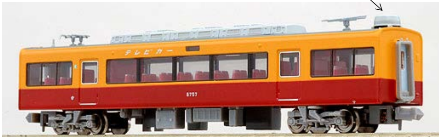
Figure 2-5 A TV-car of Keihan railway mounting a tracking antenna for BS.
