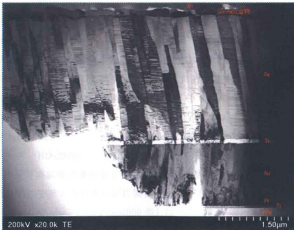
Fig. 3 TEM micrographs of AlN/Ti/Pt/Au/(Ti/Ag/Sn) thin-film multi layer ( \times 20,000 )
