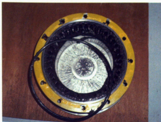
(c) 正常 WN 継手外筒
