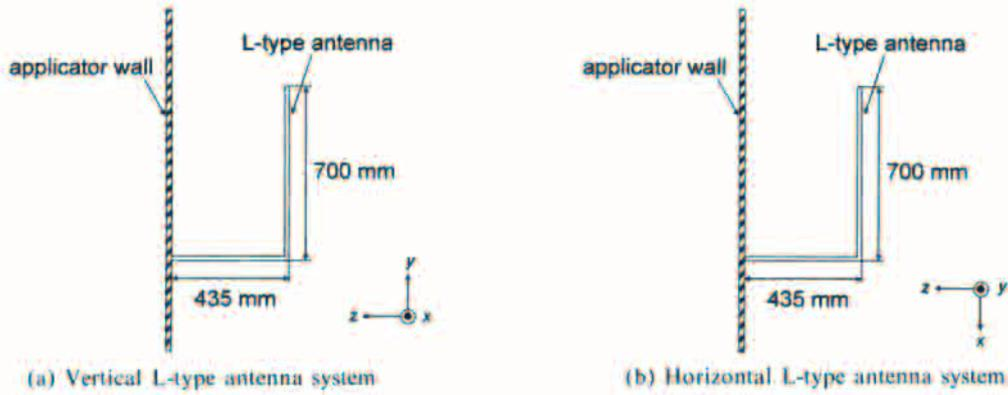
Fig. 4. Structure and setup of the L-type antenna.
