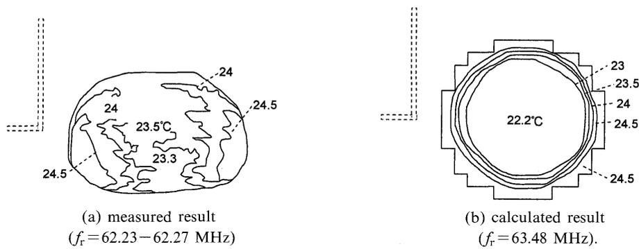
Fig. 9. Vertical L-type antenna (dotted line) was placed at  $x=-450$  mm. Measured and calculated temperature distributions on the cross section at  $x=0$  mm, where,  $T_0$  and  $T_c$  were  $21.4^\circ\text{C}$  and  $21.5^\circ\text{C}$ , respectively.
