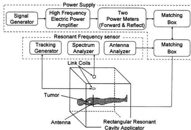
Fig. 2. Schematic of our experimental setup.
