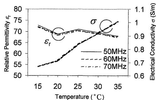
Fig. 1. Electrical constants of a torso-shaped dielectric phantom.
