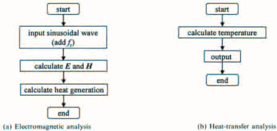
Fig. 6. Flow diagrams for electromagnetic and heat-transfer analysis.
