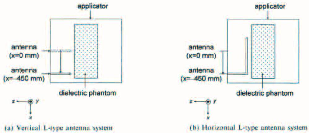
Fig. 5. Location of the L-type antenna ( $x = -450$  mm).
