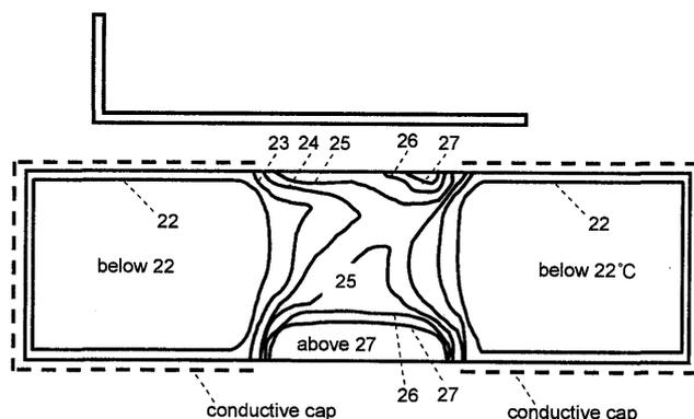
**Fig. 11.** Example for the calculated result of the dielectric phantom with conductive caps. Result shows heating distribution for the central horizontal plane of the dielectric phantom.
