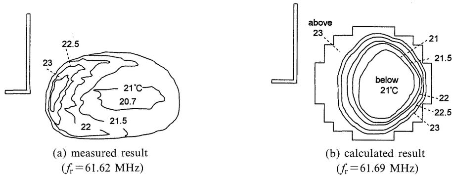
Fig. 8. Vertical L-type antenna (solid line) was placed at  $x=0$  mm. Measured and calculated temperature distributions on the cross section at  $x=0$  mm, where,  $T_0$  and  $T_c$  were  $20.5^\circ\text{C}$  and  $20.8^\circ\text{C}$ , respectively.
