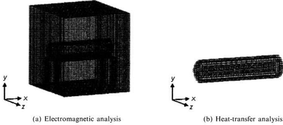
**Fig. 7.** Analytical models for electromagnetic and heat-transfer analysis.
