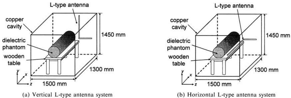
Fig. 3. Arrangement of a rectangular resonant cavity applicator.
