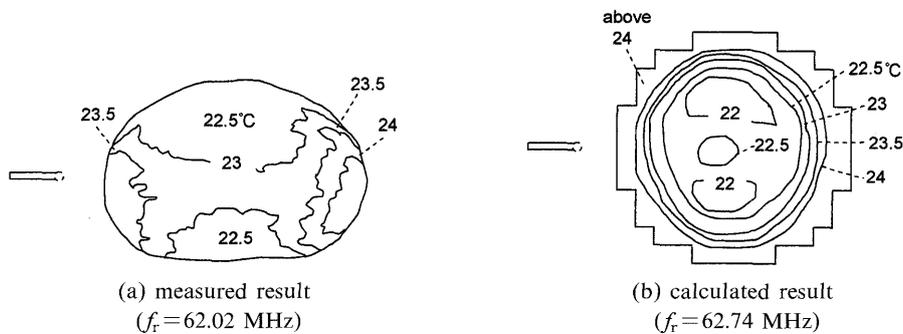
**Fig. 10.** Horizontal L-type antenna (dotted line) was placed at  $x=-450$  mm. Measured and calculated temperature distributions on the cross section at  $x=0$  mm, where,  $T_0$  and  $T_c$  were  $20.3^\circ\text{C}$  and  $20.7^\circ\text{C}$ , respectively.
