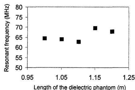
**Fig. 12.** Relationship of resonant frequency and length of the dielectric phantom, where the diameter is  $\phi 300$  mm.
