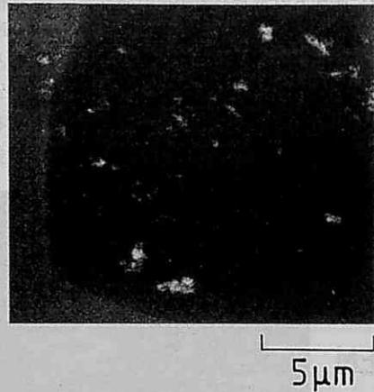
Fig. 5. TiN powder prepared by CVD at  $1550^\circ\text{C}$ .
