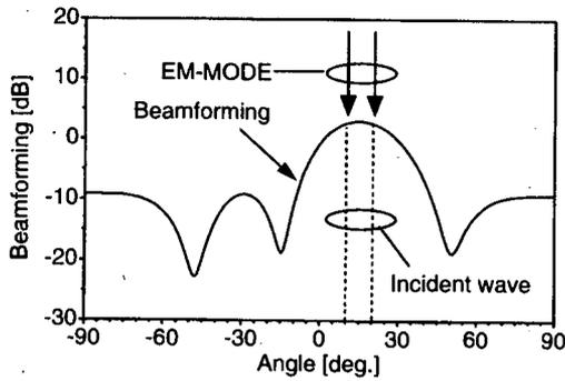
(a) DOA estimation by EM-MODE method and Beamforming
