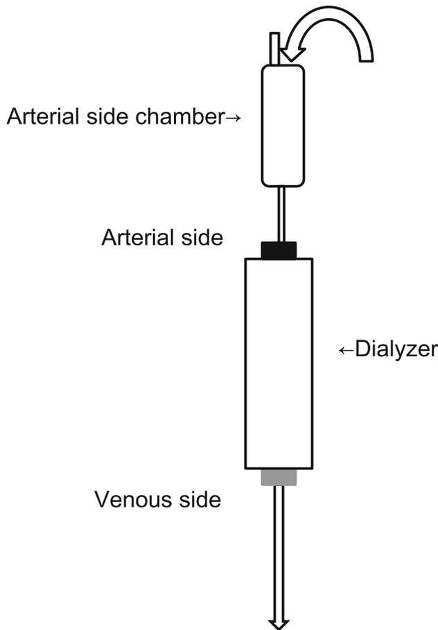
**Fig. 1** Schema of the single-pass experiment to examine nafamostat mesilate adsorption to each dialyzer
