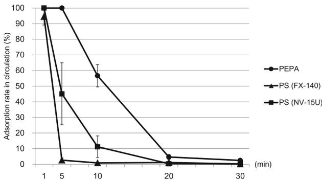
**Fig. 4** Changes of the nafamostat mesilate adsorption rate in circulation in each dialyzer ( $n = 5$ , respectively). *PEPA* polyester-polymer alloy, *PS* polysulfone
