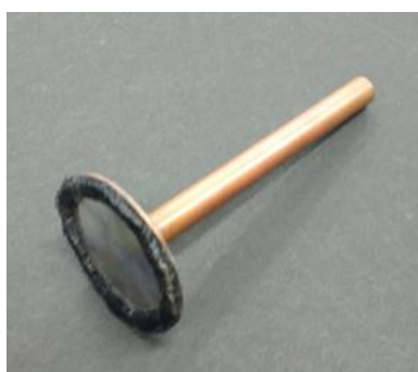
Fig. 2.5 Cold disk cathode whose diameter is 29 mm. (Reproduced from Ref. [32].)
