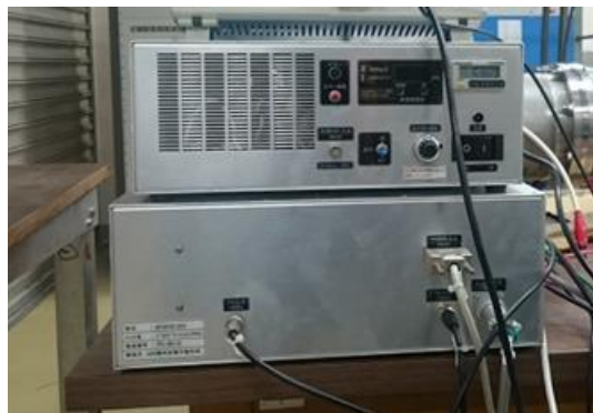
Fig. 2.4 Photo of MPC voltage supply.
