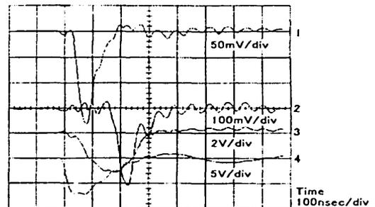
Fig.4 Time history signals: 1 prompt signal, 2 delayed signal, 3 beam current and 4 beam voltage.
