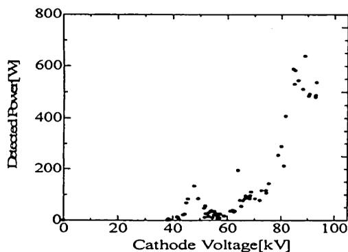
Fig.5 Output power versus the cathode voltage for K-band SWS. The magnetic field is 0.8 T.
