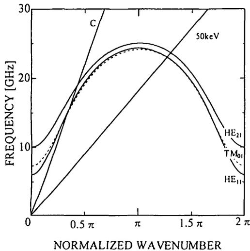
Fig.2 Dispersion curves of  $HE_{11}$ ,  $TM_{01}$ , and  $HE_{21}$ . As a reference, 50 keV beam line and light line are plotted.
