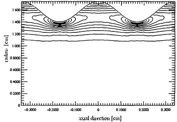
Fig.3 Distribution of  $|E|$  of  $HE_{11}$  mode in K-band SWS at the  $\pi$  point
