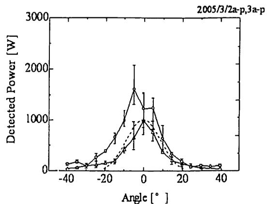
Fig.7 Example of radiation pattern for a high-power oversized BWO; with  $E_\theta$  (O) and  $E_\phi$  ( $\Delta$ ) polarization. The beam voltage and current are respectively about 90 kV and 300 A. The magnetic field is 0.8 T.
