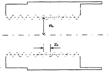
Fig.1 Schematic diagram of SWS modular used in the oversized BWO experiments. The wall radius  $R_w(z)$  varies along the axial direction  $z$  as  $R_0 + h \cos(k_0 z)$ , where  $k_0 = 2\pi/z_0$ .
