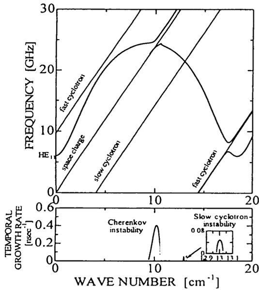
Fig.8 Dispersion characteristics of HE<sub>11</sub> mode.
