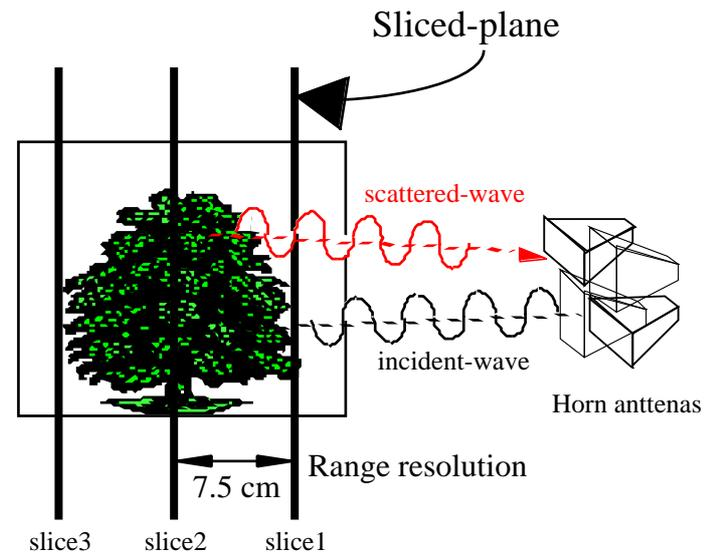
Fig.2 A geometry of sliced plane along range direction.
