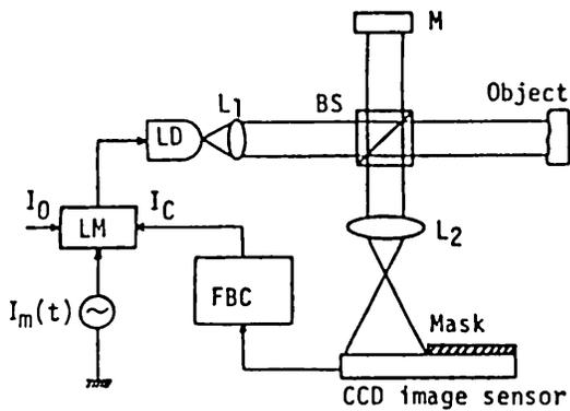
Fig.1. Phase locked laser diode interferometer.
