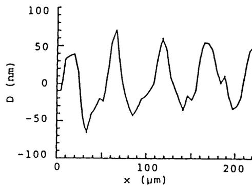
Fig.4. Measured surface profile.
