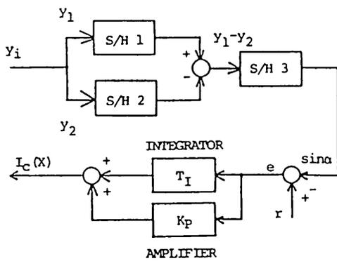
Fig.2. Block diagram of the feedback controller (FBC).
