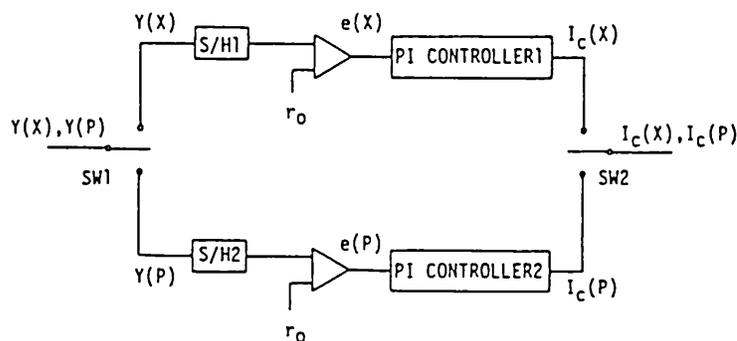
Fig.5. Block diagram of the feedback controller to eliminate external disturbance.
