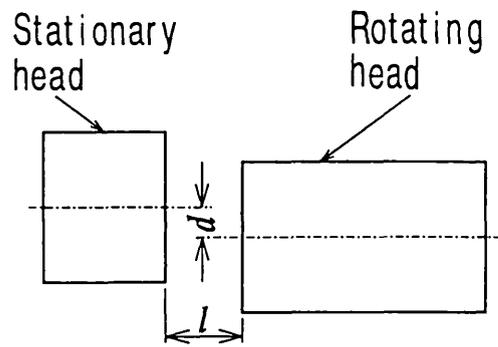
Fig.6 Relative position between the both heads.
