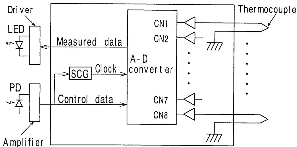
Fig.4 Block diagram of the electrical circuit in the rotating head.
