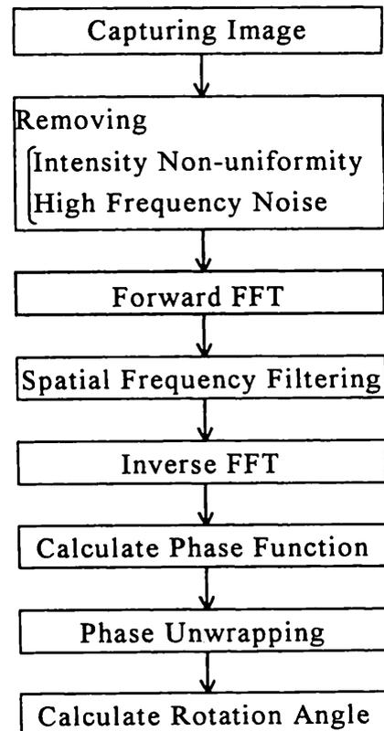
Fig. 2 Flow chart of the image processing.
