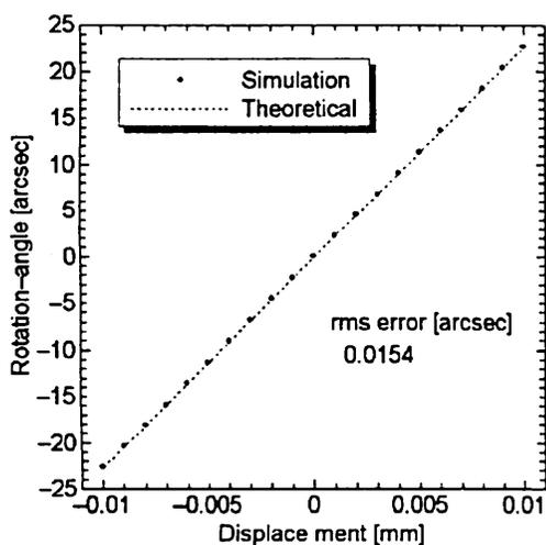
Fig. 9 Measurement error calculated by a simulation with the sinusoidal grating.
