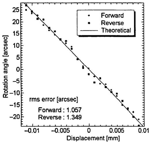
Fig. 13 Rotation angle measurement with a sinusoidal grating. Travel pitch of the micrometer-head is 1  $\mu\text{m}$ .
