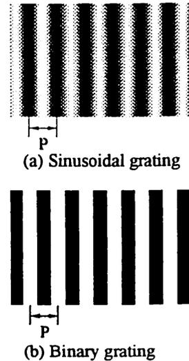
Fig. 5 Grating images used in the experiments.
