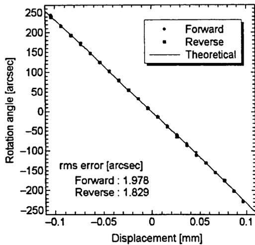
Fig. 11 Rotation angle measurement with a sinusoidal grating. Travel pitch of the micrometer-head is 10  $\mu\text{m}$ .
