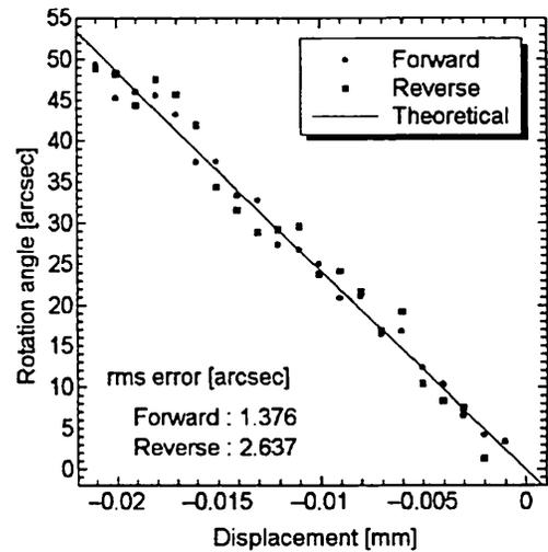
Fig. 14 Rotation angle measurement with a binary grating. Travel pitch of the micrometer-head is 1  $\mu\text{m}$ .
