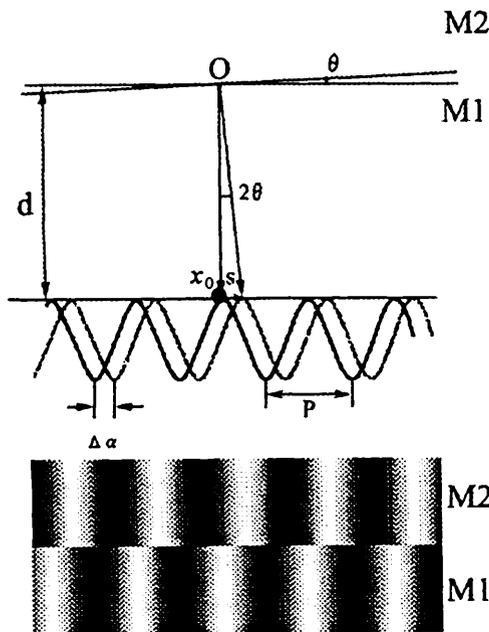
Fig. 1 Principle of the measurement. M1, Reference mirror; M2, Object mirror;  $s$ , Fringe shift;  $\Delta\alpha$ , Phase difference;  $P$ , Grating pitch;  $d$ , Viewing distance.
