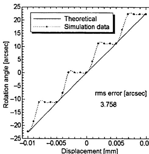
Fig. 10 Measurement error calculated by a simulation with the binary grating.
