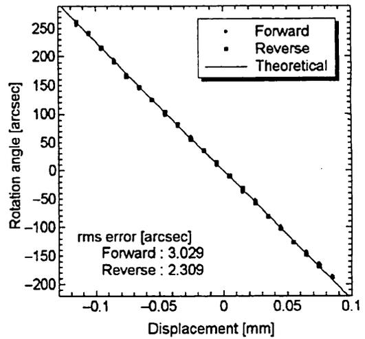
Fig. 12 Rotation angle measurement with a sinusoidal grating. Travel pitch of the micrometer-head is 10  $\mu\text{m}$ .
