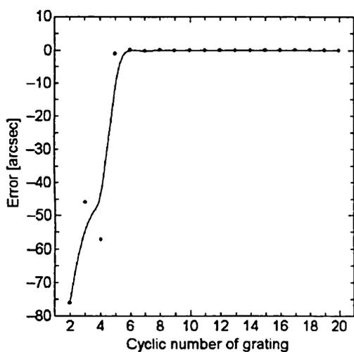
Fig. 7 Measurement error depending on the cyclic numbers of the grating.
