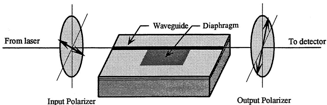
Fig.2 A sensor system using a pair of crossed polarizers to detect the induced phase difference between the two orthogonal guided modes.
