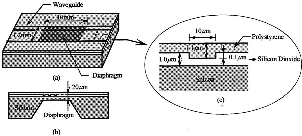
Fig.5 (a) Schematic drawing of the fabricated sensor, (b) its cross-sectional view, and (c) the cross-section of the ridge-type waveguide. The width of the polystyrene channel waveguides was  $10\ \mu\text{m}$ , and the dimensions of the diaphragm are  $1.2\ \text{mm} \times 10\ \text{mm} \times 20\ \mu\text{m}$ .
