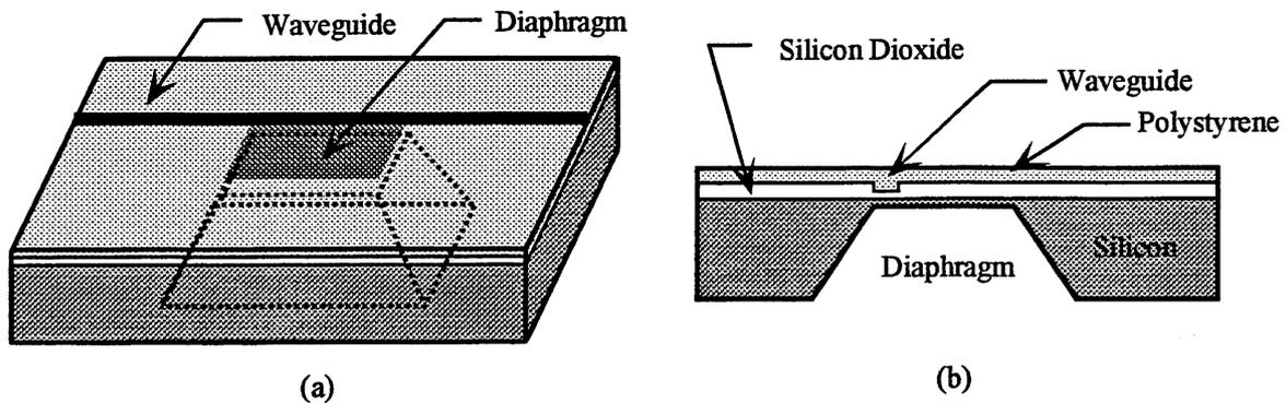
Fig.1 (a) Schematic drawing of the integrated optical pressure sensor using intermodal interference, and (b) a cross-sectional view.
