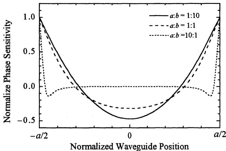
Fig.4 The relations between the normalized phase sensitivity and the waveguide position in the  $y$ -direction. The waveguide positions of  $\pm a/2$  represent the waveguide along the side of the diaphragm, whereas a position of 0 corresponds to the center of the diaphragm.
