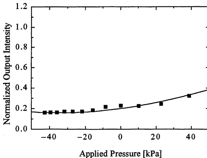
Fig.7(b) The experimental result for the waveguide apart from the waveguide of Fig.7(a) by 0.2 mm inside the diaphragm. The phase sensitivity was 13 mrad/kPa, corresponding to a halfwave pressure of 240 kPa.
