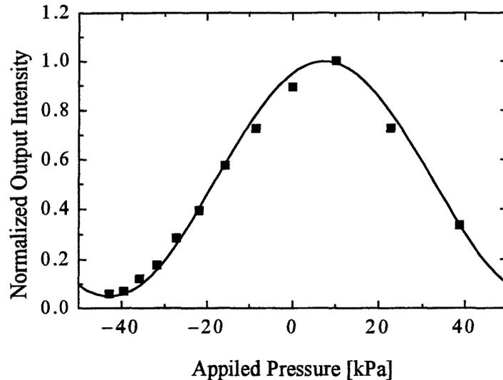
Fig.7(c) The experimental result for the waveguide apart from the waveguide of Fig.7(a) by 0.55 mm inside the diaphragm. The waveguide position was almost center since the diaphragm width was 1.2 mm. The phase sensitivity was 63 mrad/kPa, corresponding to a halfwave pressure of 50 kPa
