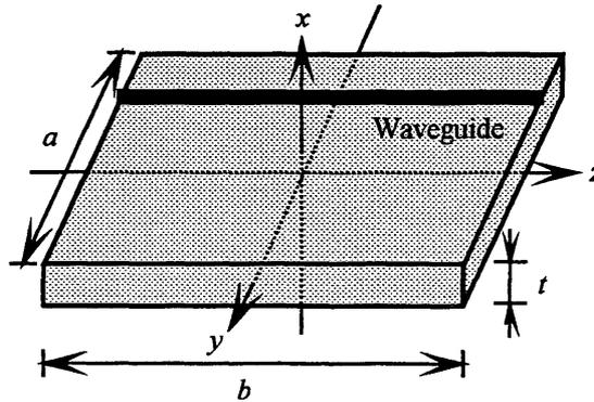
Fig.3 Illustration of the rectangular diaphragm assumed in the calculations.
