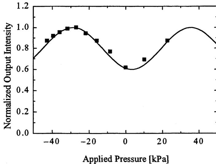
Fig.7(a) The experimental result and the best fit sinusoidal curve for the waveguide nearest to the diaphragm edge. The phase sensitivity was 98 mrad/kPa, corresponding to a halfwave pressure of 32 kPa.
