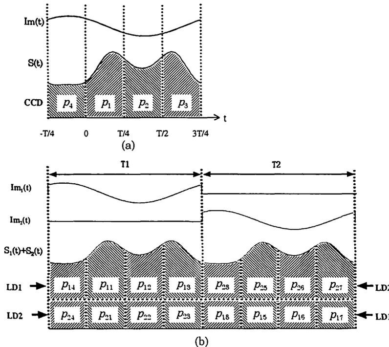
Fig. 2 Integrating-bucket method with (a) the ordinary modulating technique and (b) the time-shared sinusoidal phase modulation.
