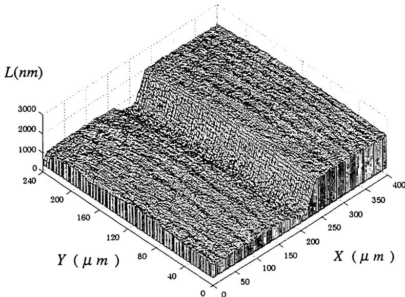
Fig. 4 Measurement result of the step-height of  $1\mu\text{m}$ .
