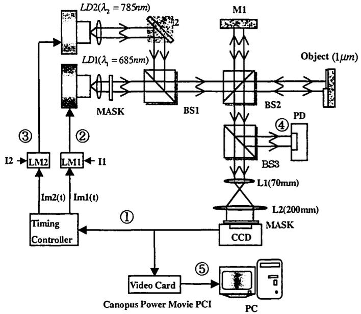
Fig. 1 Experimental setup of two-wavelength laser diode interferometer using time-sharing sinusoidal phase modulation.
