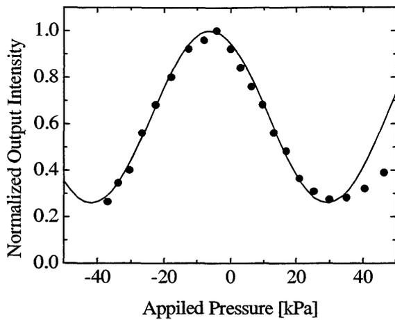
Fig. 6(a) The experimental result of normalized output intensity versus applied pressure for the waveguide nearest to the diaphragm edge.
