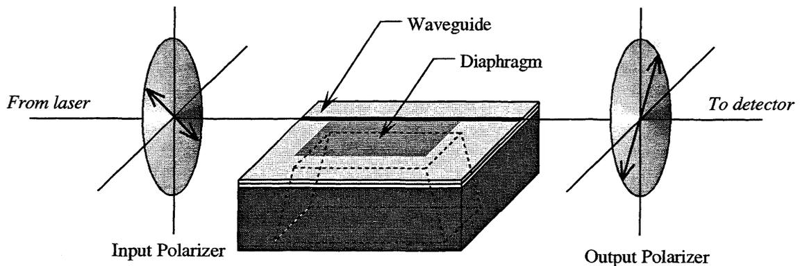
Fig. 2 A sensor system including a pair of crossed polarizers.
