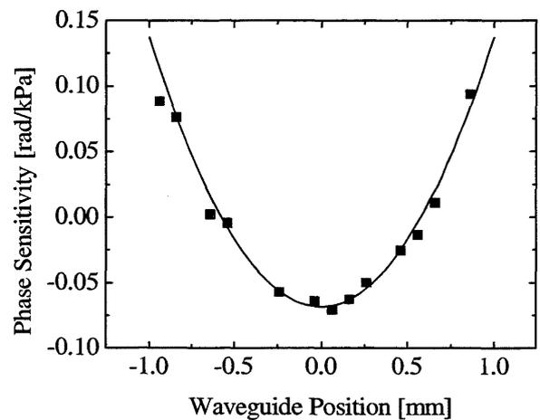
Fig. 7 Measured sensitivity as a function of the waveguide position on the diaphragm.
