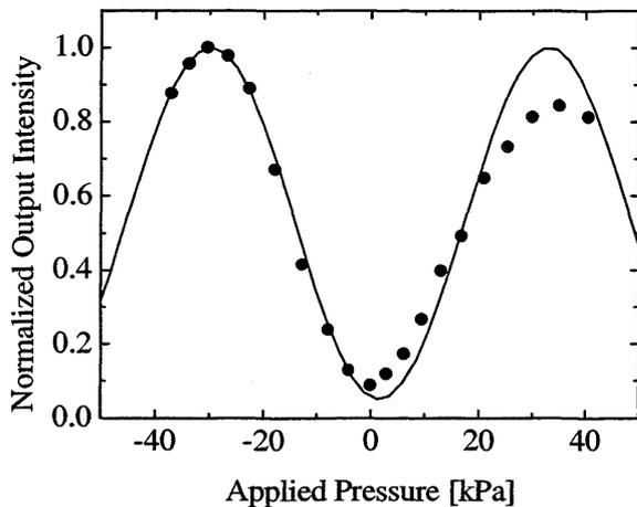
Fig. 8(a) The experimental result of normalized output intensity versus applied pressure for the waveguide nearest to the diaphragm edge.
