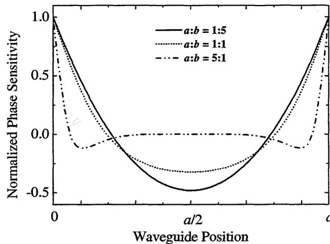
Fig. 3 Relationships between normalized phase sensitivity and waveguide position. Waveguide positions of 0 and  $a$  represent that the waveguide is placed along the edge of the diaphragm, whereas a position of  $a/2$  corresponds to the center of the diaphragm.
