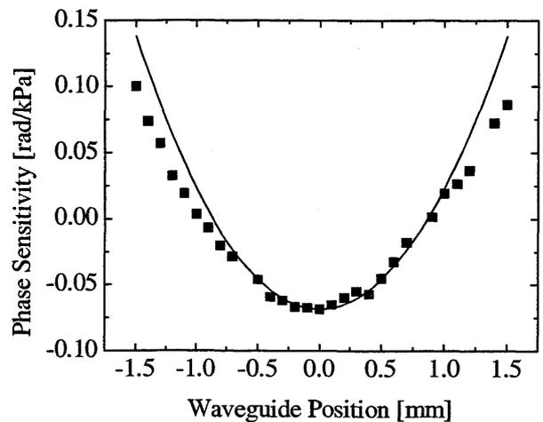
Fig. 9 Measured sensitivity as a function of the waveguide position on the diaphragm.
