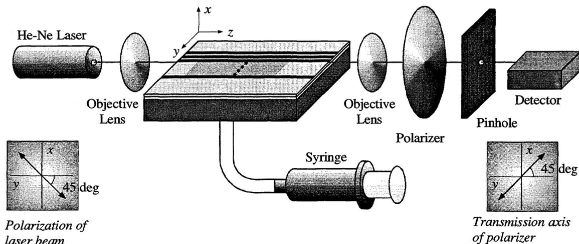
Fig. 5 The arrangement of the sensor system to measure the output intensity as a function of the applied pressure.
