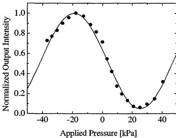
Fig. 6(c) The experimental result for the waveguide located 1.0 mm from the waveguide of Fig. 6(a). The waveguide is the nearest to the center of the diaphragm.
