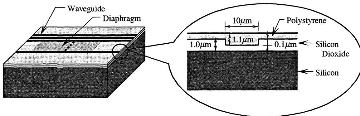
Fig. 4 Schematic drawing of the fabricated sensor and the cross-section of the waveguide. The width of the polystyrene channel waveguides was  $10 \mu\text{m}$ , and the diaphragm dimensions of two fabricated sensors are (1)  $2.0 \text{ mm} \times 10 \text{ mm} \times 35 \mu\text{m}$  and (2)  $3.0 \text{ mm} \times 15 \text{ mm} \times 64 \mu\text{m}$ .
