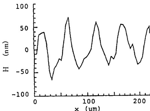
Fig. 10 1-D surface profile measured with PLLD interferometer.
