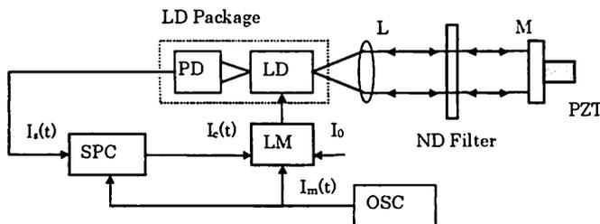
Fig. 6 Self-mixing type of LD interferometer.
