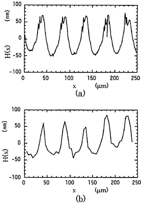
Fig. 13 1-D surface profile measured with (a) Talystep profiler and (b) differential type of PLLD interferometer.
