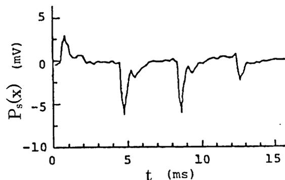
Fig. 11 Temporal change of the feedback signal in PLLD interferometer.
