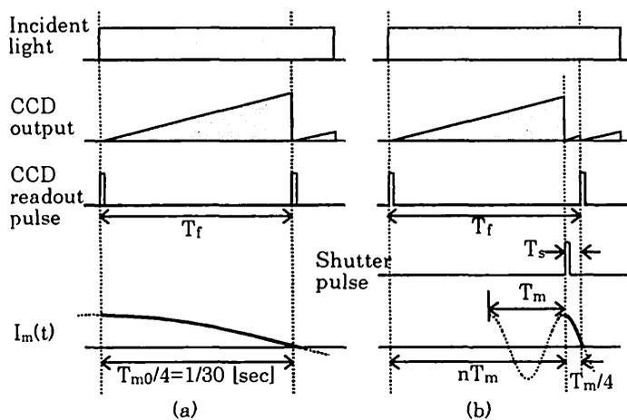
Fig. 20 Schematic of (a) a conventional; modulating signal and (b) a high-speed modulating signal.
