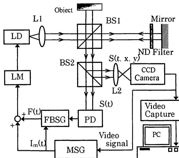
Fig. 19 Disturbance-free high-speed SPM LD interferometer.
