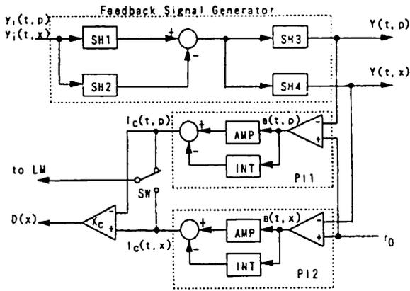
Fig. 12 Differential type of PLLD interferometer.
