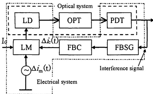
Fig. 1 Feedback type of laser diode interferometer.
