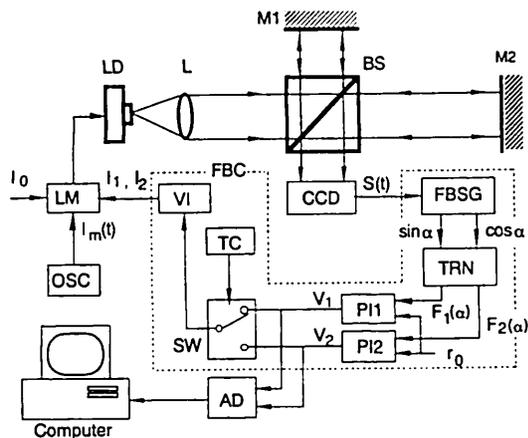
Fig. 14 Wavelength multiplexed LD interferometer for distance measurement.
