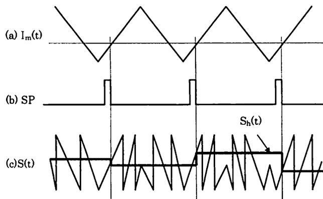
Fig. 7 Schematic of the FB signal generation by use of the sampling technique .
