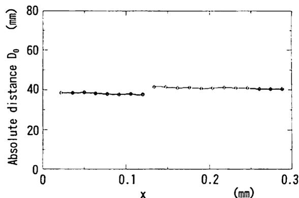
Fig. 16 Measured step-height of the gauge block whose thickness was  $\sim 2$  mm.
