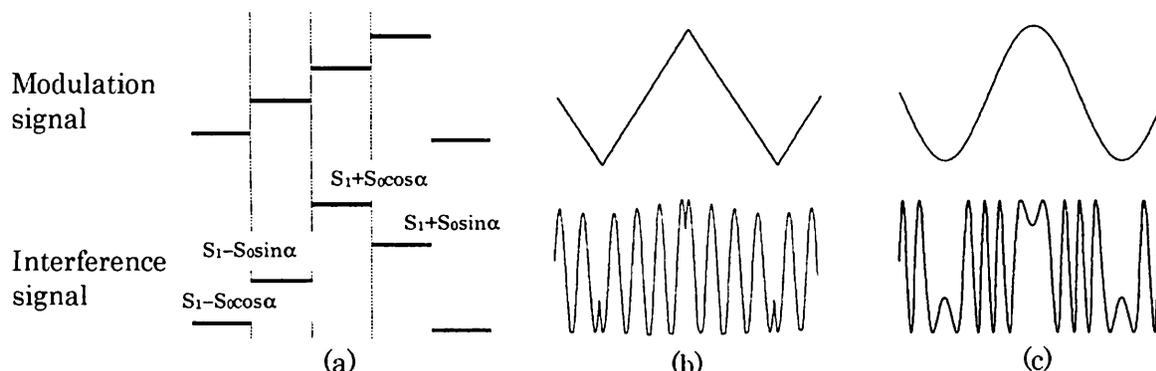
**Fig. 3** Interferometries classified by the modulation signal: (a) phase shifting LD interferometry, (b) heterodyne LD interferometry, and (c) sinusoidal phase modulating LD interferometry.
