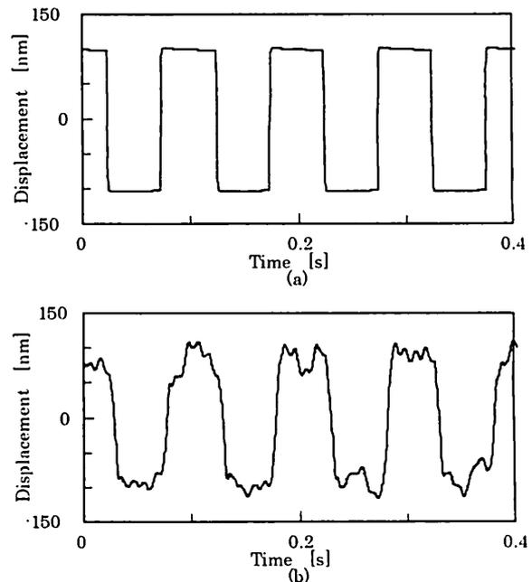
Fig. 8 Rectangular-displacements (a) calculated with the PZT's driving signal and (b) measured with self-mixing LD interferometer.
