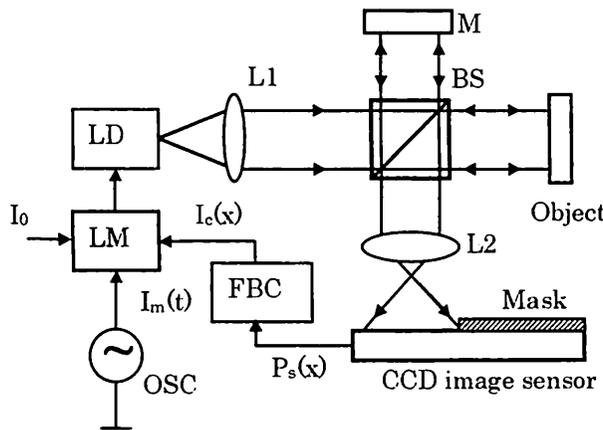
Fig. 9 Phase-locked laser diode interferometer.
