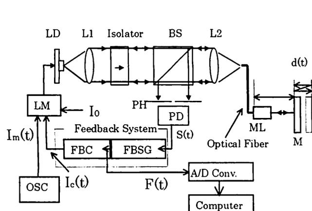
Fig. 4 Setup for the displacement measurement.
