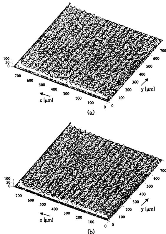
Fig. 21 3-D surface profile of a diamond-turned aluminum disk. Profile (b) was measured 10 min after the first measurement shown in (a).
