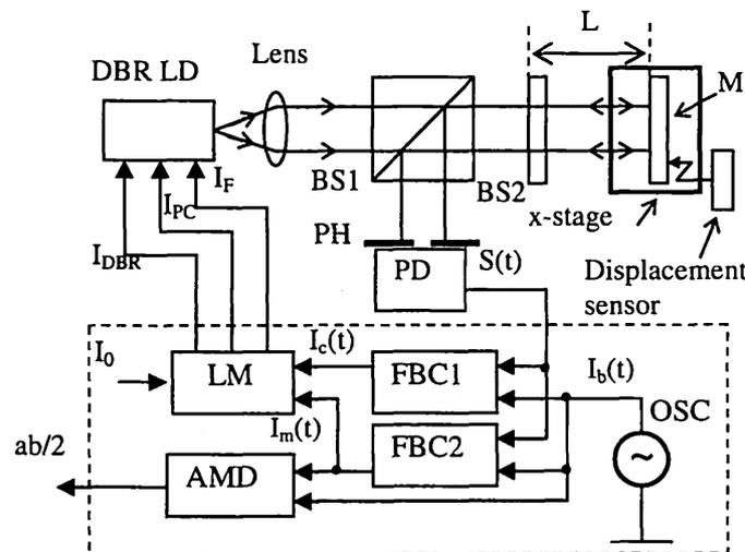
Fig. 1 Experimental setup: PH, pinhole; PD, photodiode; LM, laser modulator; FBC, feedback controller; OSC, oscillator; AMD, amplitude detector.
