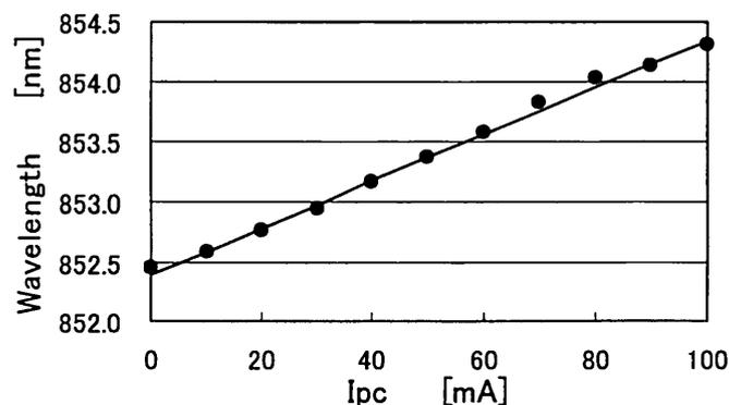
Fig. 6 DBR LD wavelength change according to  $I_{PC}$ . The ratio between  $I_{PC}$  and  $I_{DBR}$  is 1:1.4.
