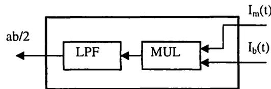
Fig. 2 Block diagram of the AMD: MUL, multiplier; LPF, low-pass filter.
