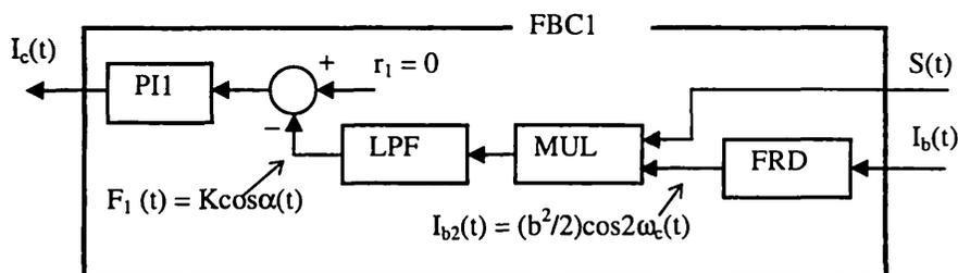
Fig. 3 Block diagram of the FBC1: FRD, frequency doubler; PI1, proportional-integral controller.
