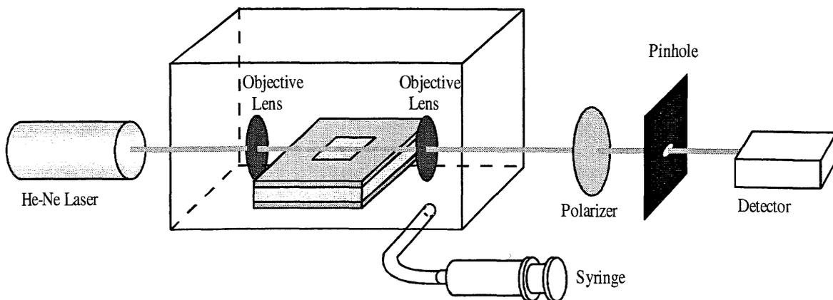
Fig. 8 Experimental setup to measure output intensity as a function of applied pressure. A sensor and two objective lenses were put in a closed box.
