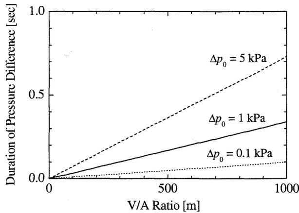
Fig. 4 Duration of the induced pressure difference as a function of the V/A ratio. In the figure, the initial pressure difference is taken as a parameter.
