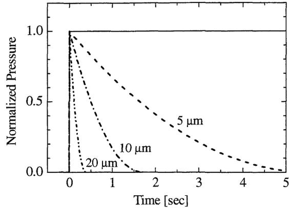
Fig. 3 Normalized pressure difference  $\Delta p(t)/\Delta p_0$  induced on the diaphragm as a function of time; diameter of the small hole is taken as a parameter. In the figure, the solid line represents the ambient pressure change.
