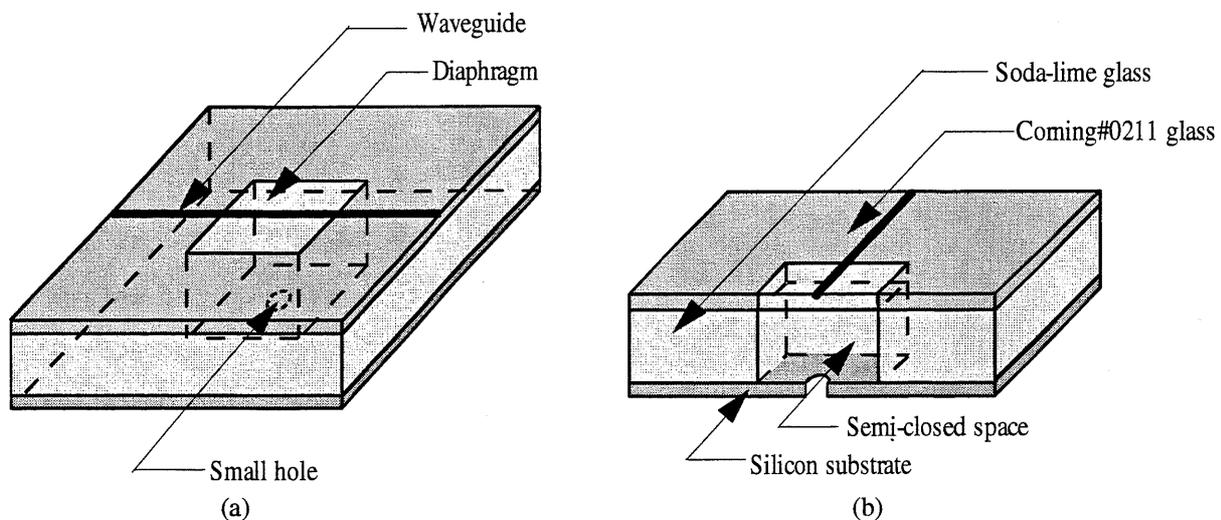
Fig. 1 (a) Schematic drawing of a guided-wave optical pressure sensor using intermodal interference. The sensor shows a response only to sudden pressure change by a semi-closed space with a small hole. (b) The cross-sectional view of the sensor.
