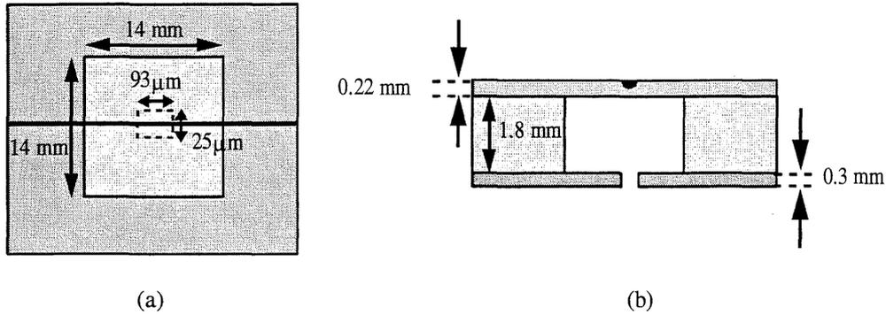
Fig. 5 (a) Top and (b) cross-sectional views of the fabricated sensor and actual dimensions.
