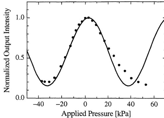
Fig. 7 Normalized output intensity versus applied pressure for the waveguide nearest to the center of the diaphragm.
