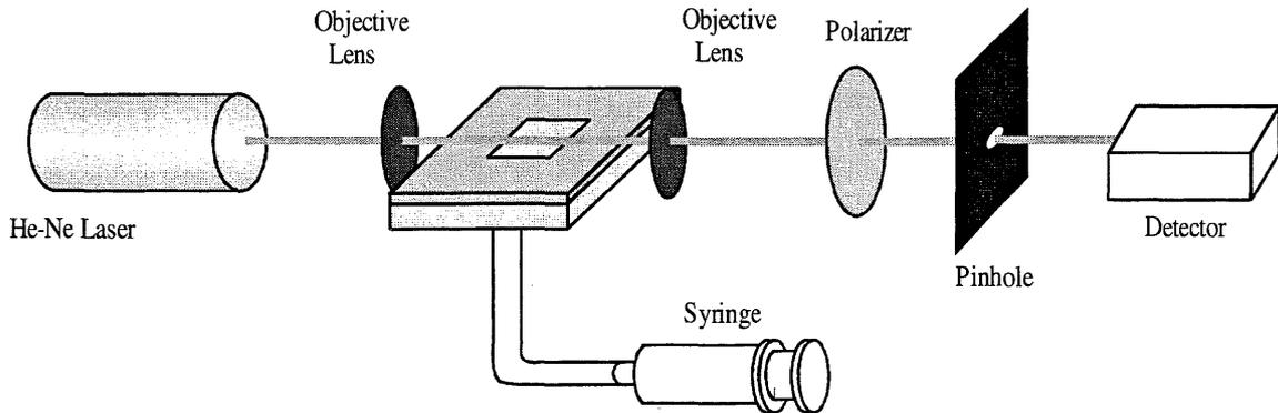
Fig. 6 Experimental setup to measure output intensity as a function of applied pressure.
