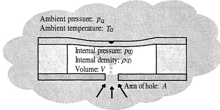
Fig. 2. Schematic diagram mathematically showing how the sensor obtains the induced pressure difference and its duration. In the model, the volume of the semi-closed space is  $V$ , and the sectional area of the small hole is  $A$ . The pressure and temperature in the surroundings just after the sudden pressure change are  $p_a$  and  $T_a$ , respectively. The pressure and density in the semi-closed space are  $p(t)$  and  $\rho(t)$ , respectively.
