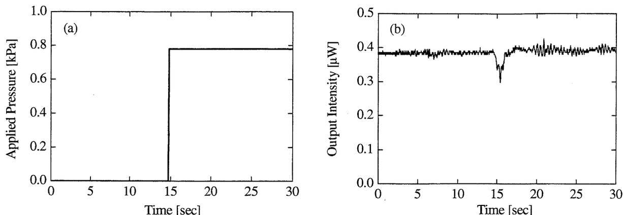
Fig. 9 (a) Ambient pressure change was increased by 0.78 kPa in a stepwise fashion at about 15 sec. (b) Measured output intensity as a function of time.
