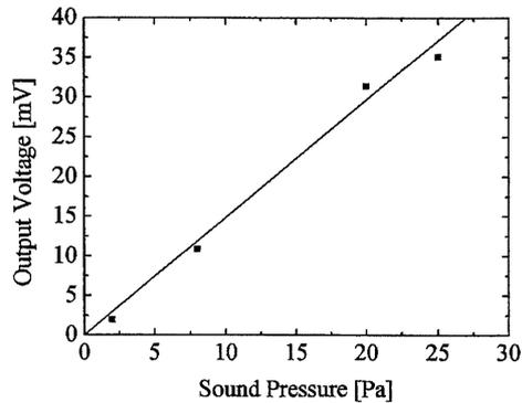
Fig 12 The net microphone output versus sound pressure
