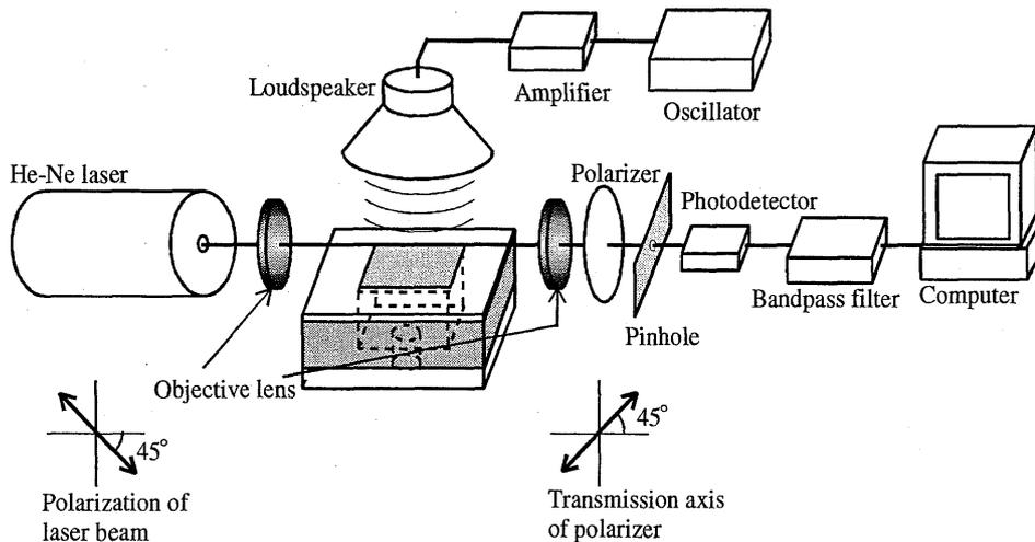
Fig. 7 Experimental setup to measure the output power as a function of the applied sound pressure.
