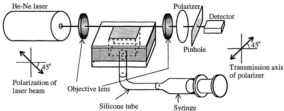
Fig. 5 Experimental setup used to evaluate phase sensitivity.
