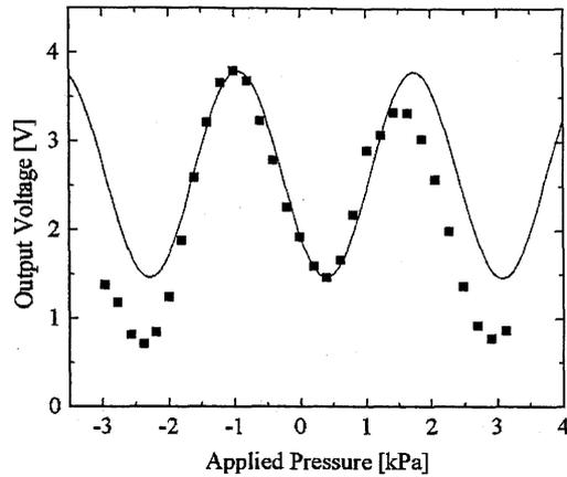
Fig. 6 Output voltage of the photodetector versus applied pressure.
