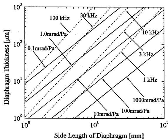
Fig. 3 Theoretical trajectories of equal sensitivities and equal resonance frequencies on the side length - thickness plane.
