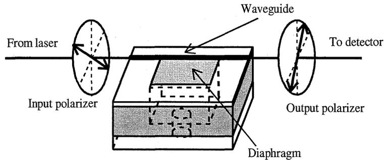
Fig. 2 Schematic diagram of a guided-wave optical microphone placed between a pair of crossed polarizers.
