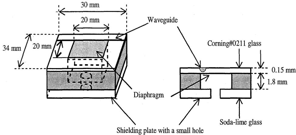
Fig. 4 Schematic diagram of the fabricated optical microphone with actual dimensions.
