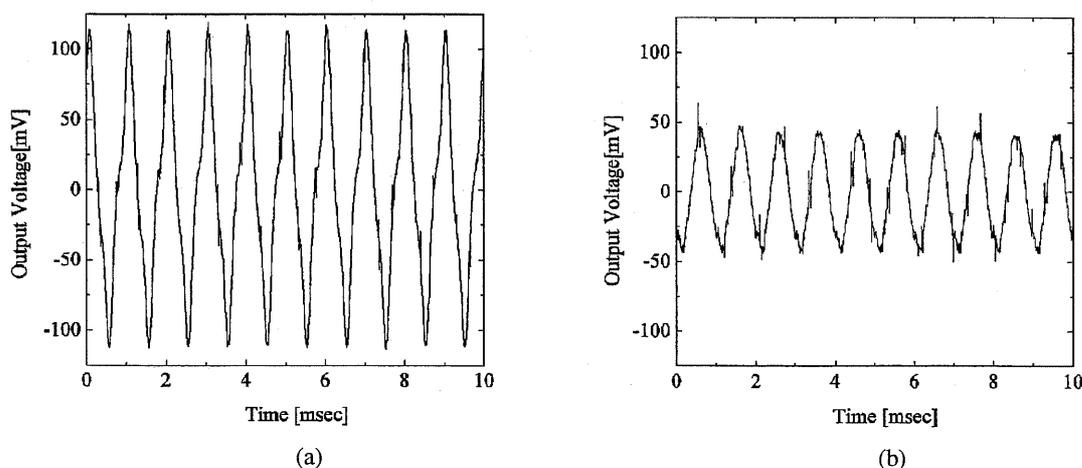
Fig. 8 (a) A nominal microphone signal (with the output polarizer), and (b) a misalignment signal (without the output polarizer) responding to a sound wave of 25 Pa and 1 kHz.
