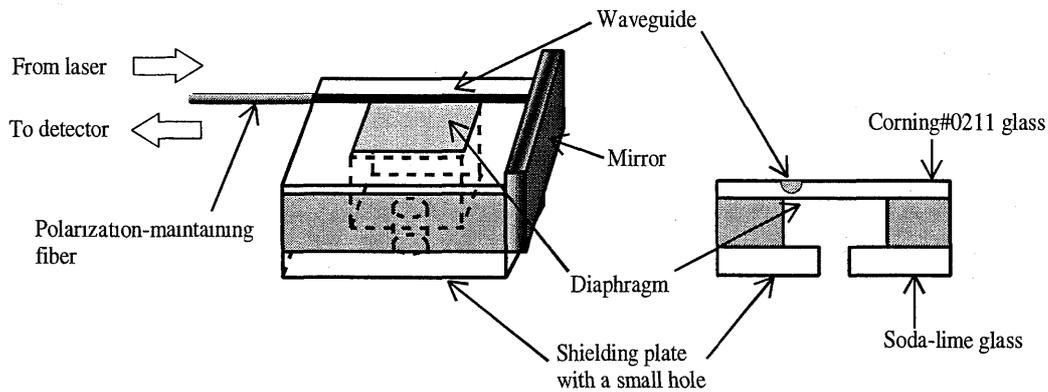
Fig 1 Schematic drawing of a glass-based guided-wave optical microphone.
