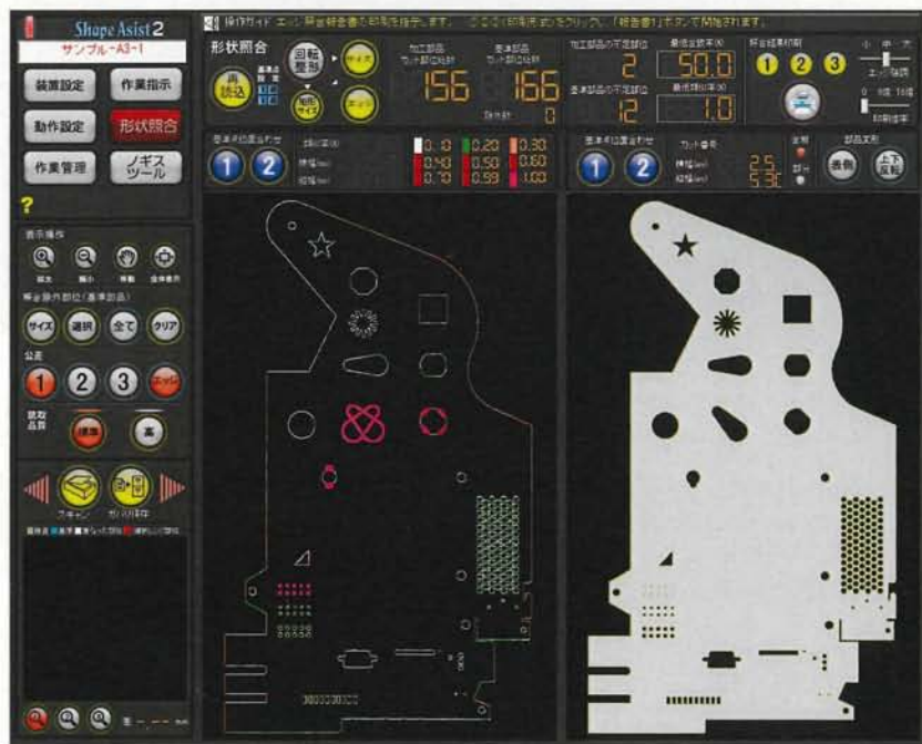
Fig. 20 Matching process between the converted edge image and original DXF image.
