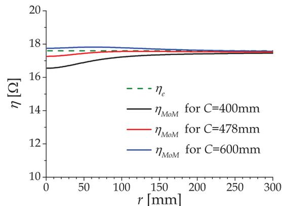
Fig. 4. Distance Dependence of Simulated Wave Impedance of the Insulated Circular Loop Antenna (ICLA) with the circumference of  $C = 400$  mm, 478 mm, and 600 mm in the Tissue-Equivalent Liquid at 30 MHz
