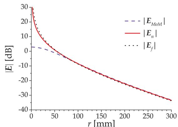
Fig. 6. Distance Dependence of three types of Simulated Electric Field Intensity,  $|E_{MoM}(r)|$ ,  $|E_n(r)|$ , and  $|E_f(r)|$ , of the Insulated Circular Loop Antenna (ICLA) with the circumference of  $C = 478$  mm in the Tissue-Equivalent Liquid at 30 MHz
