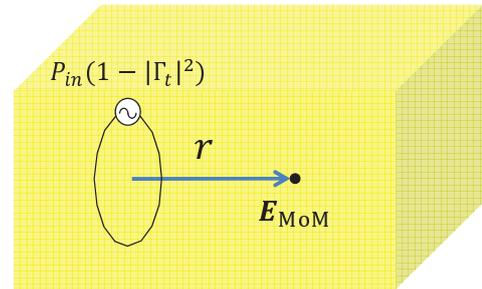
Fig. 2. Geometry for Calculating Electric Field Intensity Radiated by an Insulated Circular Loop Antenna (ICLA) by Richmond's code
