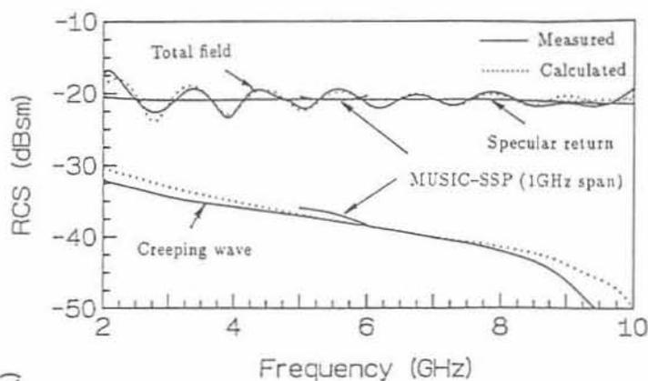
Fig.1. The backscattered total, specular, and creeping fields for a 101.6mm $\phi$  metal sphere. MUSIC-SSP(1GHz span) denotes the extracted results by eq.(6).
