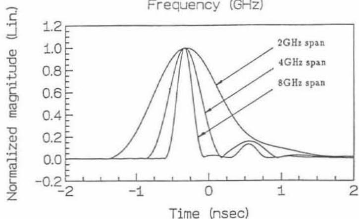
Fig.2. Time-domain responses of a 101.6mm $\phi$  metal sphere using the inverse-FFT. 2GHz span : The swept frequency band is from 4.5GHz ~ 6.5GHz. 4GHz span : The swept frequency band is from 3.0GHz ~ 7.0GHz. 8GHz span : The swept frequency band is from 2.0GHz ~ 10.0GHz.
