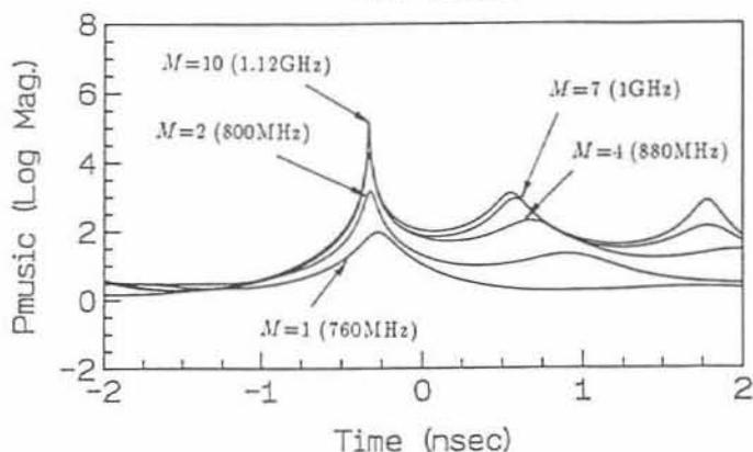
Fig.3. Scattering center estimation of a 101.6mm $\phi$  metal sphere using the MUSIC-SSP.  $N=20$ ,  $f_1=5.0\text{GHz}$ ,  $\Delta f=40\text{MHz}$ . The value in the parenthesis ( ) denotes the required frequency bandwidth.
