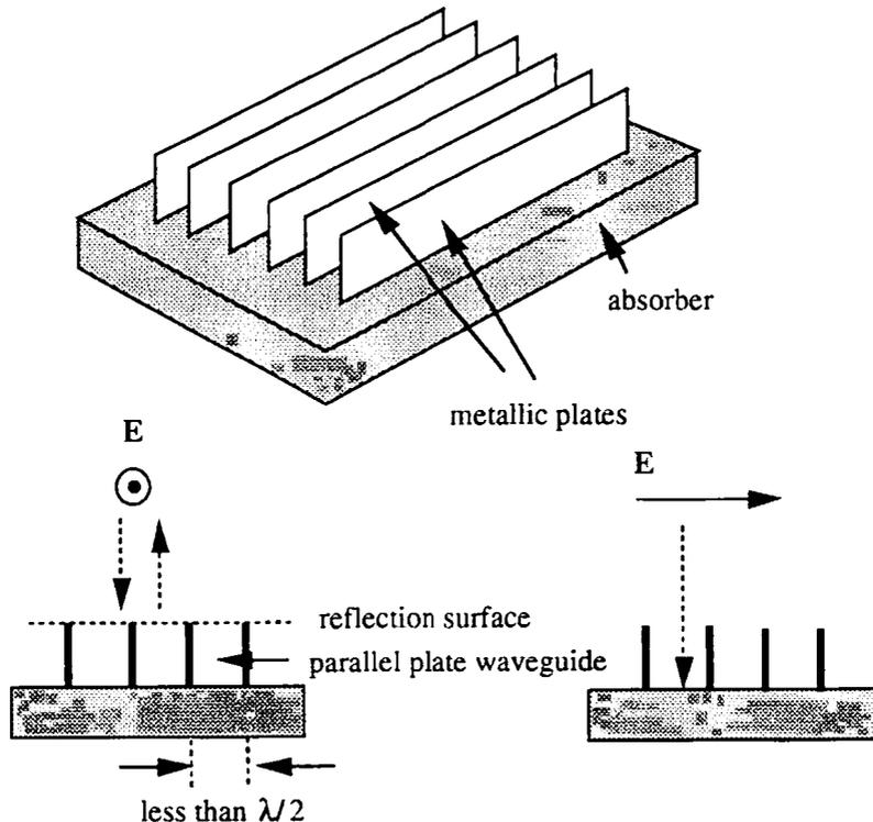
Fig.1 A proposed linear target for the calibration.
