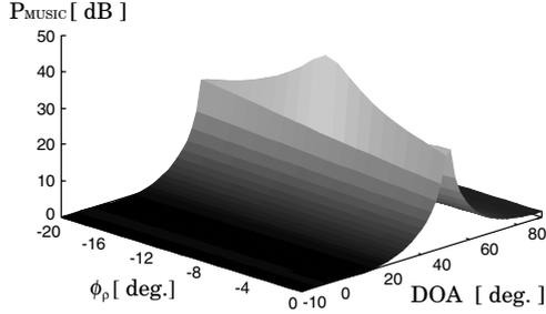
Fig. 2: DOA and Calibration coefficient estimation by  $P_{\text{MUSIC}}(\theta, \phi_\rho)$ .  $N = 4$ ,  $\Delta x_1 = \Delta x_2 = \Delta x_3 = 0.48\lambda$ ,  $\theta_0 = 50^\circ$ ,  $\text{SNR} = \infty$ (no noise).
