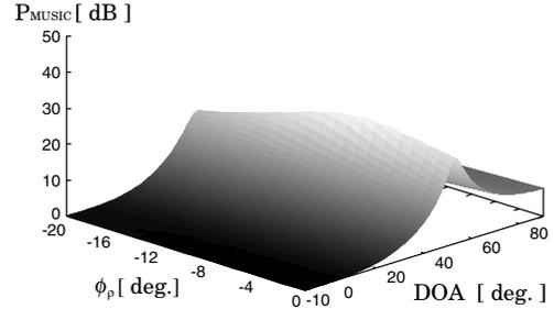
Fig. 4: DOA and Calibration coefficient estimation by  $P_{\text{MUSIC}}(\theta, \phi_\rho)$ .  $N = 4$ ,  $\Delta x_1 = \Delta x_2 = \Delta x_3 = 0.2\lambda$ ,  $\theta_0 = 50^\circ$ ,  $\text{SNR} = \infty$ (no noise).
