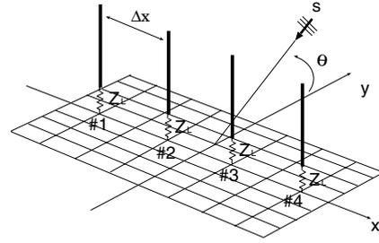
**Fig. 7:** DOA estimation with 4-element monopole array
