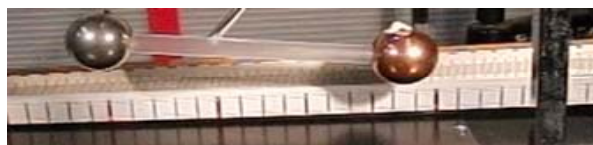
FIGURE 7. Movie of high speed camera for 2 body pendulums (made of steel and brass) collisions in CMS.
