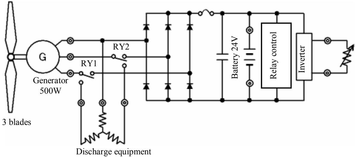
Fig.1. Control system of the micro wind turbine.
