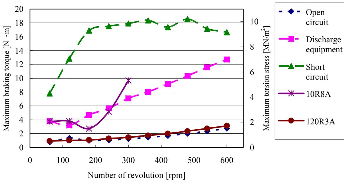
Fig.9. Maximum braking torque and Maximum torsion stress.
