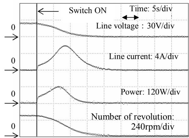
Fig.6. An example of waveforms (10R8A at 300 rpm).
