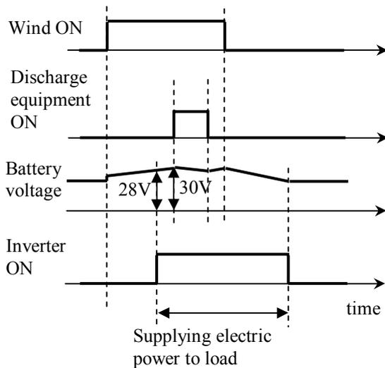
Fig.2. Control device operation.
