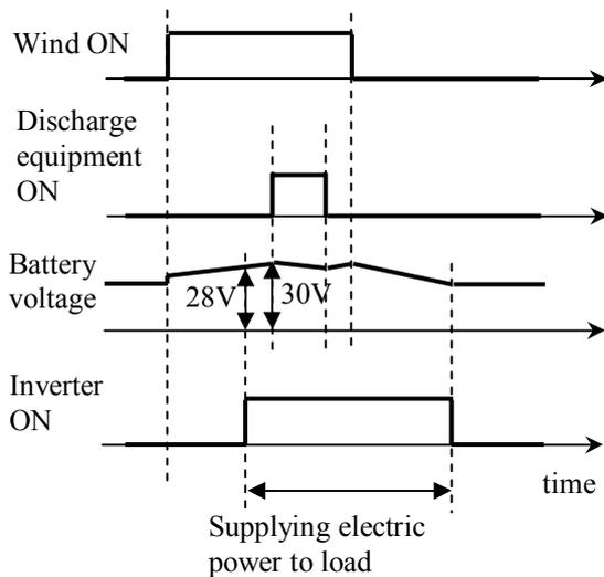
Fig.2. Control device operation.
