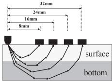
Fig.9 Expected optical path in the two-layered specimen
