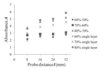
Fig. 7 Relation between the probe distance l and the absorbance A for the two-layered specimens with respect to the measured water content. The results of the single layered specimens are also shown
