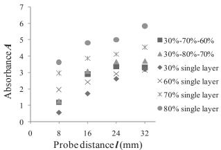
Fig.8 Relation between the probe distance l and the absorbance A for the three-layered specimens with respect to the measured water content. The results of the single layered specimens are also shown
