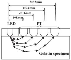
Fig.2 Schematic of change of NIR light paths in gelatin specimen with distance *l* between LED and PT
