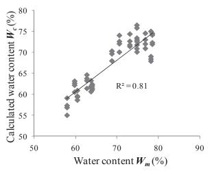
Fig.6 Relation between the measured water content  $W_m$  and the calculated water content  $W_C$  for the single layered specimens
