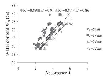
Fig.5 Relation between the NIR absorbance A and the measured water content  $W_m$  for the single layered specimens with respect to the probe distance l
