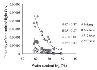
Fig.3 Relation between the measured water content  $W_m$  and the intensity of transmitted light I for the single layered specimens with respect to the probe distance l. The intensity I is represented by electrical current
