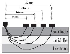
Fig.10 Expected optical path in three-layered specimen
