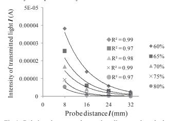
Fig.4 Relation between the probe distance l and the intensity of transmitted light I for the single layered specimens with respect to the measured water content  $W_m$ . The intensity I is represented by electrical current
