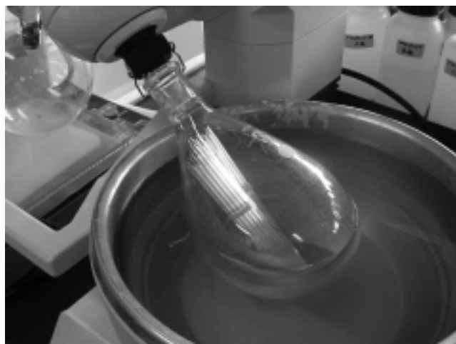
Fig.3. Evaporation of water in Kjeldahl digested solution in Pyrex glass tubes by round bottom flask with short neck.
