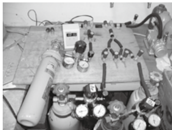
Figure 2 Photograph of vacuum system for exchanging the gas in test tubes.
