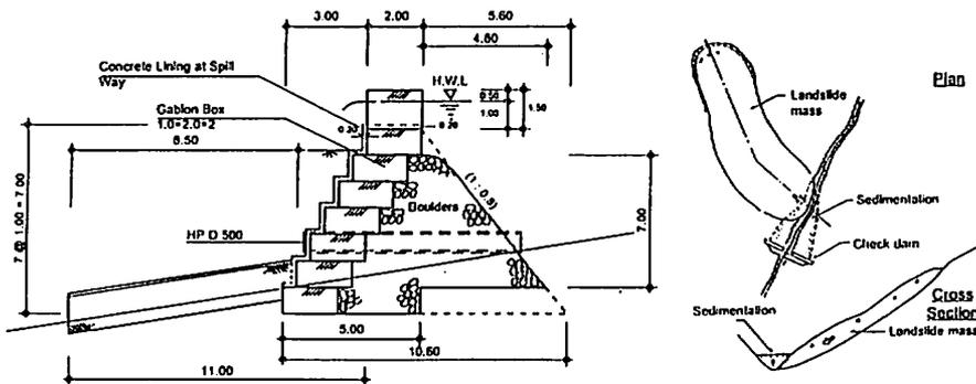
**Figure 5 :** Consolidation dam applied to act as toe loading at the foot of landslide block.
