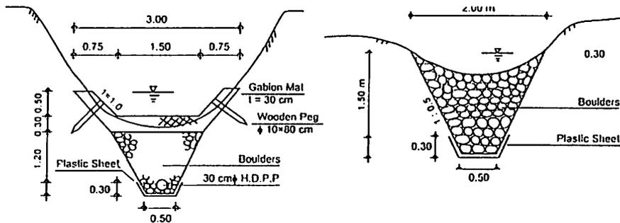
**Figure 4 :** Various types of surface drainage works tried to reduce the construction cost, utilizing local material
