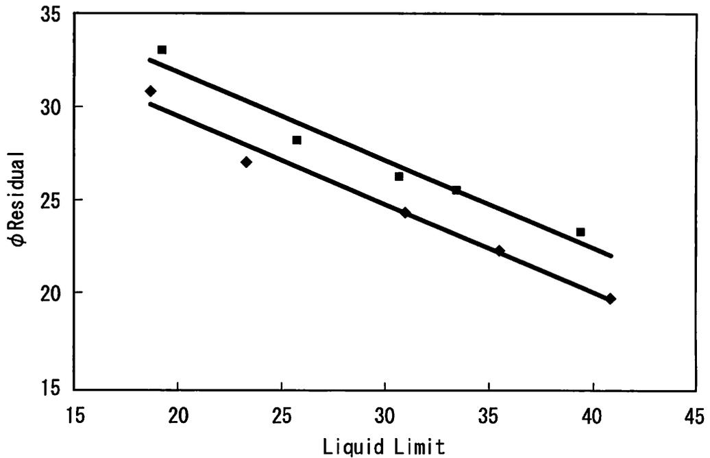
Figure 2 : Relationship between liquid limit and residual  $\phi$ .
