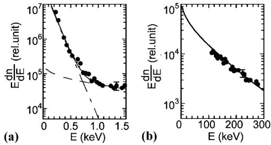
FIG. 3. (a) An x-ray energy spectrum in the central cell obtained by the ULE Ge detector is fitted by the theoretical curve (the solid curve) calculated using two-component Maxwellian electron distribution function. (b) An x-ray spectrum from higher-energy component is also observed by a NaI(Tl) detector.
