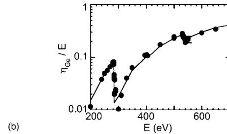
FIG. 2. (a) Schematic drawings of the experimental apparatus in TERAS. (b) The quantum efficiency of the ULE Ge detector normalized by the incident x-ray energy. The theoretical curve (the solid line) is calculated based on the x-ray absorptions by a specially fabricated polymer window.
