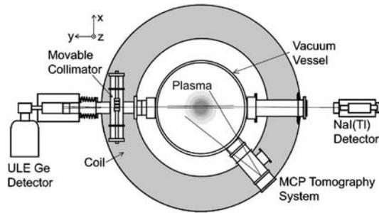
FIG. 1. Schematic drawings of x-ray diagnostic systems in the central cell of GAMMA 10.
