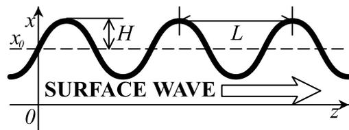
Fig. 1 Analytical model. The SWS is the metal surface which is corrugated sinusoidally in the  $z$ -direction.  $H$  and  $L$  are the ripple amplitude and the period of the corrugation, respectively.
