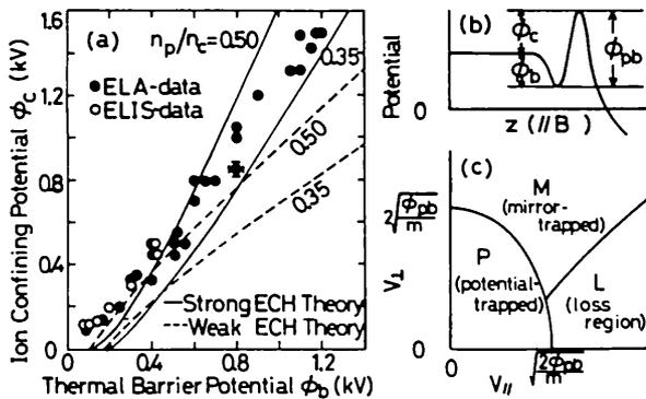
FIG. 1. (a) Scaling data on  $\phi_c$  vs  $\phi_b$  as compared with the ECH theories. (b) An axial potential profile. (c) A model of an electron velocity distribution function due to the strong ECH theory. (Velocity space at the plug.)
