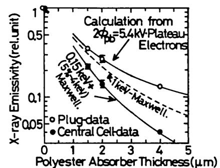
FIG. 4. X-ray tomography data ( $r=0$ ) in the plug (O) (see Fig. 3) and in the central cell (●) are compared during the thermal-barrier period. Here,  $h\nu \geq 80$  eV.
