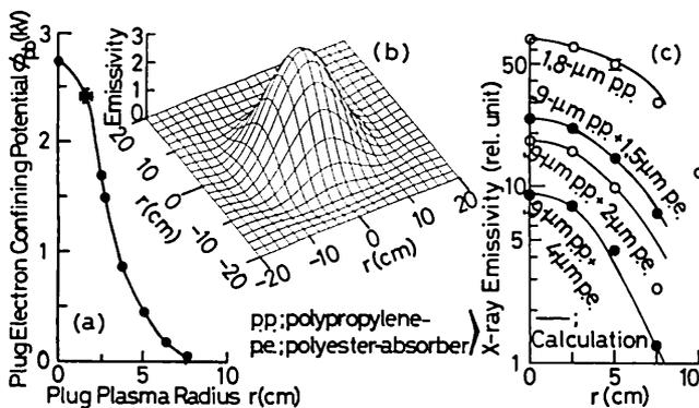
FIG. 3. (a) Radial profile data on  $\phi_{pb}$ . (b) Tomographic-reconstructed x-ray emissivity using a 1.8- $\mu\text{m}$  polypropylene absorber ( $h\nu \geq 80$  eV). (c) X-ray radial profile data with various absorbers are compared with the calculated x-ray profiles from the plateau electron distribution functions using the  $\phi_{pb}$  data in (a).
