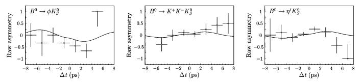
FIG. 3. The  $\Delta t$  asymmetry, A, in each bin for  $B^0 \rightarrow \phi K_S^0$  (left),  $B^0 \rightarrow K^+ K^- K_S^0$  (center), and  $B^0 \rightarrow \eta' K_S^0$  (right), respectively. The curves, which originate from time-dependent asymmetries given by  $-\xi_f S \sin(\Delta m_d \Delta t) - \xi_f A \cos(\Delta m_d \Delta t)$ , show the results of the unbinned-maximum likelihood fit.
