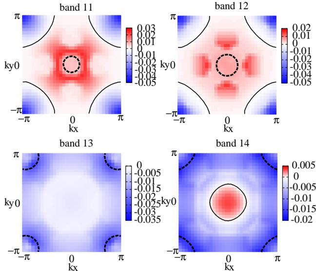
Figure 2: The gap function in the band representation for the bands from 11th to 14th near the Fermi level for  $U' = 0.756$  eV and  $J = 0.3$  eV at  $x = 0.1$  and  $T = 0.02$  eV. Solid and dashed lines represent the nodes of the gap function and the Fermi surfaces, respectively.
