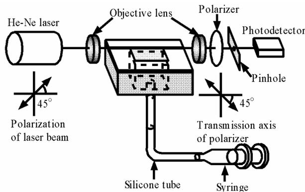
Fig. 4. Experimental setup for measuring the output intensity versus the pressure in the guided-wave optical pressure sensor.
