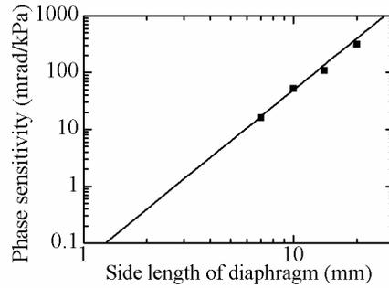
Fig. 6. Sensitivity dependence on the side length of the diaphragm for the waveguide nearest to the center of the diaphragm. Dots show the measured sensitivities of Sensors #1-4. Solid line shows the calculated sensitivity as a function of the side length.
