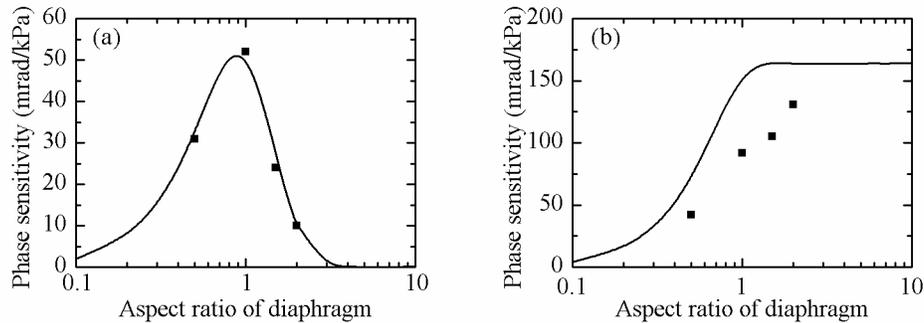
Fig. 9. Sensitivity dependence on the aspect ratio of the diaphragm for two waveguide positions: (a) nearest to the center and (b) nearest to the edge. Dots show the measured sensitivities of Sensors #2 and #5-7. Solid lines show the calculated sensitivities as a function of the aspect ratio.
