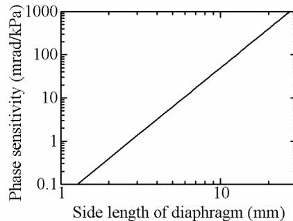
Fig. 2. Phase sensitivity as a function of the side length of the diaphragm for the waveguide on the center of the diaphragm.
