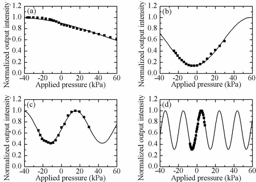
Fig. 5. Normalized output intensity versus applied pressure for the waveguide nearest to the center of the diaphragm. Figures (a)-(d) are for Sensors #1-4, respectively.
