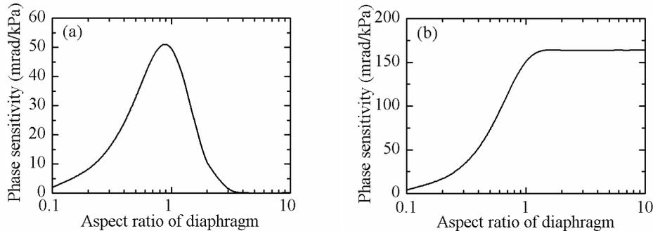
Fig. 3. Phase sensitivity as a function of aspect ratio of the diaphragm for the waveguides along (a) the center and (b) the edge of the diaphragm.
