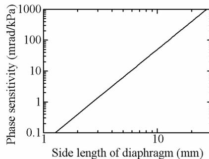
Fig. 2. Phase sensitivity as a function of the side length of the diaphragm for the waveguide on the center of the diaphragm.
