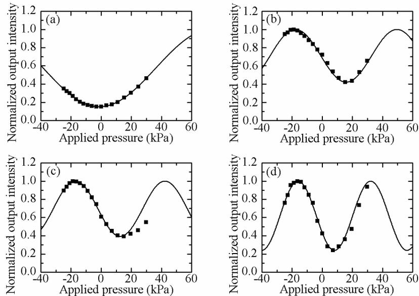
Fig. 8. Normalized output intensity versus applied pressure for the waveguide nearest to the edge of the diaphragm. Figures (a)-(d) are for Sensors #5, #2, #6, and #7, respectively.
