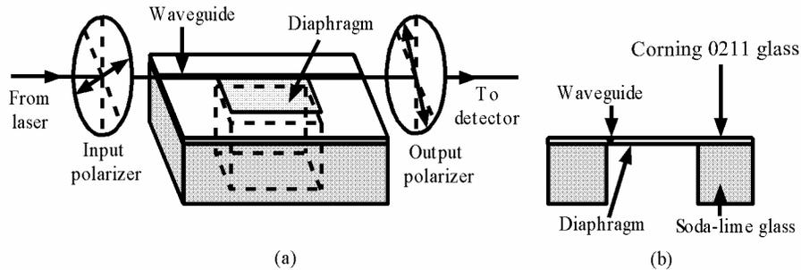
Fig. 1. (a) Configuration of the glass-based guided-wave optical pressure sensor placed between a pair of crossed polarizers and (b) its cross-section drawing.
