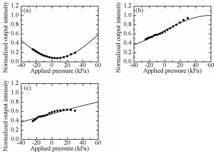
Fig. 7. Normalized output intensity versus applied pressure for the waveguide nearest to the center of the diaphragm. Figures (a)-(c) are for Sensors #5-7, respectively.
