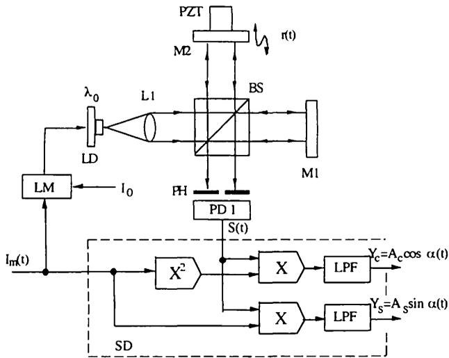
Fig. 1 SPM laser diode interferometer and a synchronous detector.
