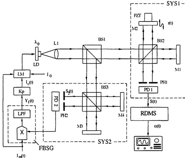
**Fig. 6** Experimental setup of the real-time displacement measurement system with feedback control.
