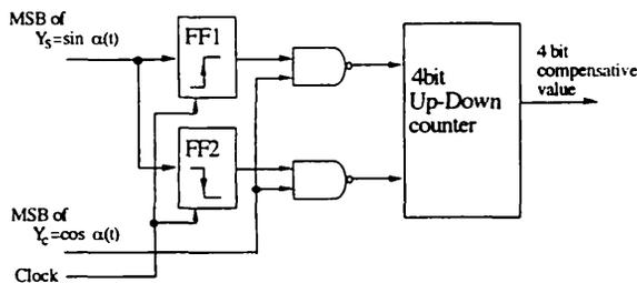
Fig. 4 Block diagram of the phase compensation circuit.
