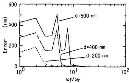
**Fig. 5** The rms error calculated from the difference between original sinusoidal vibration  $r(t)$  and detected vibration  $r'(t)$ . The horizontal axis shows the ratio between the vibrating frequency and the cutoff frequency of the LPF.
