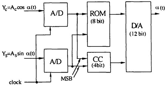
Fig. 2 Block diagram of real-time phase detector.
