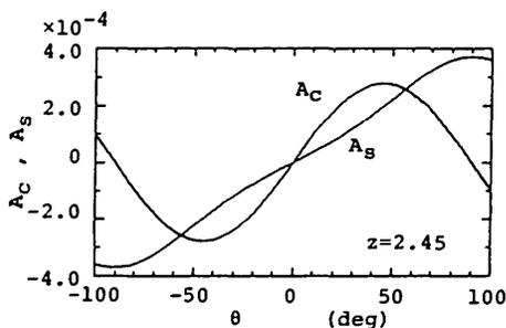
Fig. 3 Amplitudes of  $\cos\alpha(x,y)$  and  $\sin\alpha(x,y)$  calculated from Eqs. (8) and (9) for  $-100 \text{ deg} \leq \theta \leq 100 \text{ deg}$ , where  $z$  was selected as an optimum value 2.45.
