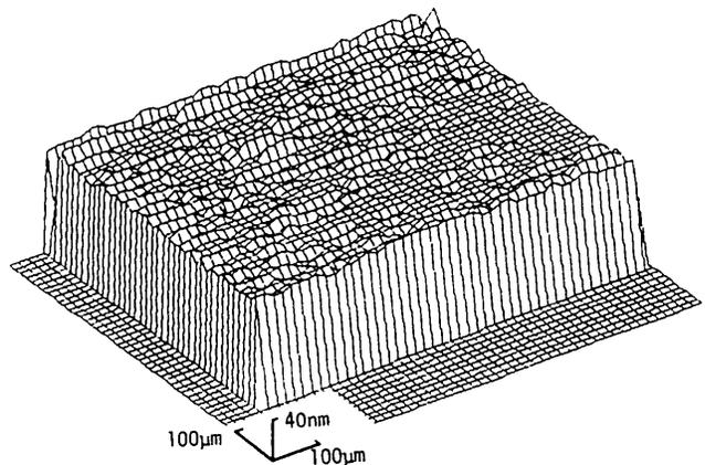
Fig. 7 Surface profile of the mirror measured by our system in real time.
