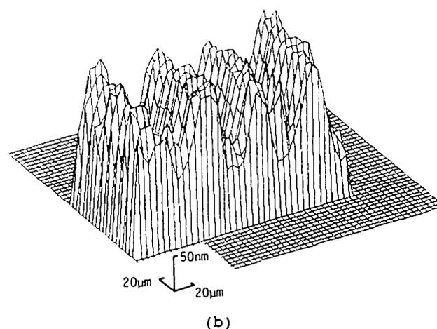
Fig. 9 Experimental results measured by our system: (a) surface profile of the same disk shown in Fig. 8 and (b) surface profile ob-
