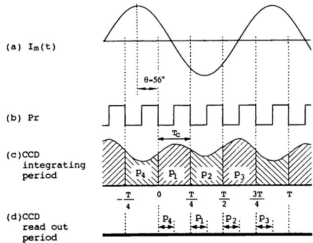
Fig. 2 Readout timing for the CCD image sensor: (a) modulation signal  $I_m(t)$ ; (b) reference pulse (Pr), which is delayed by 56 deg in phase; (c) the integrating period of the CCD image sensor homeomorphic to Pr; and (d) the readout period of the CCD image sensor.
