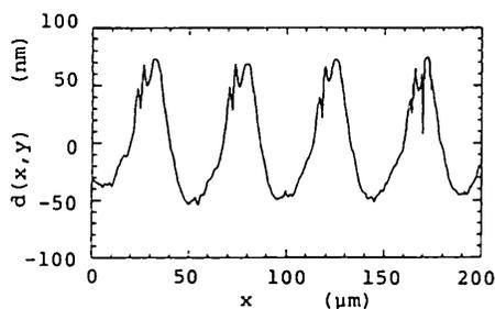
Fig. 8 Surface profile of a diamond-turned aluminium disk measured by a Talystep instrument.
