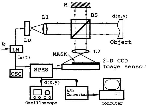
Fig. 1 Experimental setup of an SPM LD interferometer for real-time 2-D surface profile measurement. The surface profile  $d(x,y)$  of the object is calculated from the interference signal by an SPMS.
