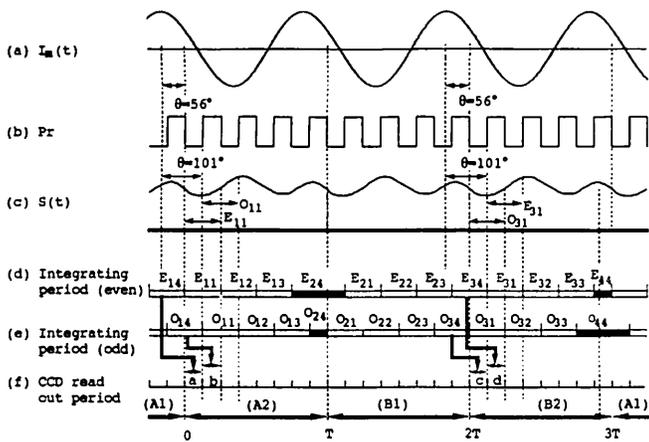
Fig. 6 Control timing of the CCD image sensor: (a) modulation signal  $I_m(t)$ ; (b) reference pulse Pr; (c) interference signal  $S(t)$ ; (d) and (e) the integrating period for even and odd field, respectively; and (f) the readout period of the CCD image sensor. The surface profiles for even and odd field are detected in the regions of (A2) and (B2), respectively.
