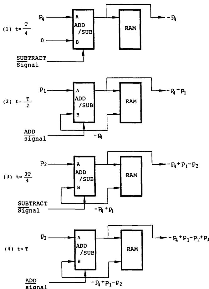
Fig. 5 Explanation of the operations in the SPMS. A cycle of the operation begins with  $p_4$  and ends with  $p_3$  to avoid the overflow.
