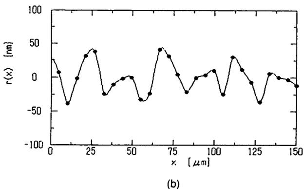
Fig. 5 Surface profiles of a diamond-turned aluminum disk measured with the position error (a)  $\Delta l = 0.4$  mm and (b)  $\Delta l = -0.4$  mm.
