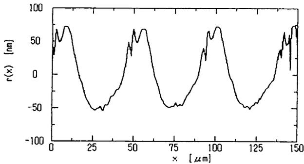
Fig. 4 Surface profile of a diamond-turned aluminum disk measured with a Talystep instrument.
