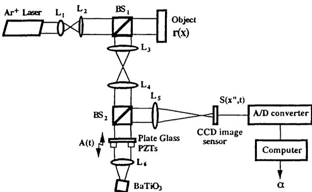
Fig. 1 SPM Fizeau interferometer using a self-pumped phase conjugator.
