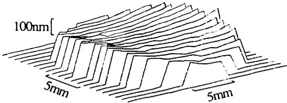
Fig. 8 Surface profile of a mirror measured with the position error  $\Delta l = 5$  mm.
