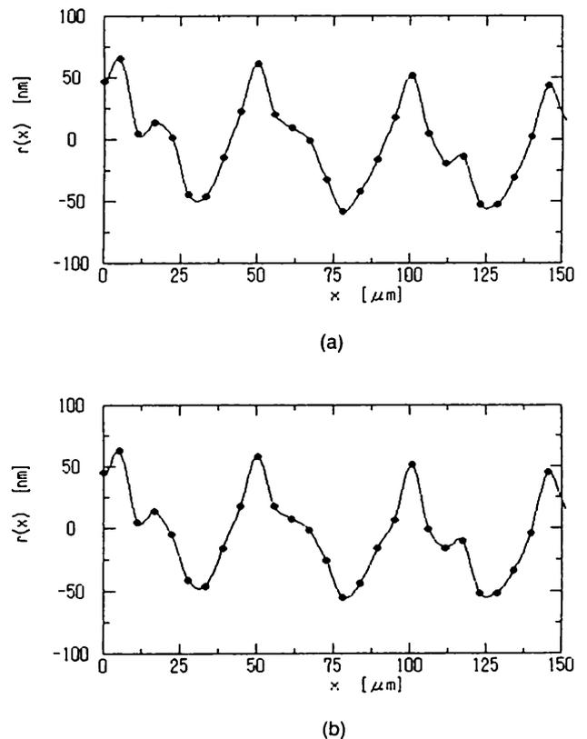
Fig. 3 (a) Surface profile of a diamond-turned aluminum disk. (b) The same surface disk measured after interval of a few minutes.
