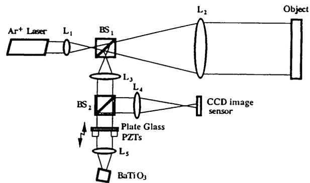
Fig. 6 SPM Fizeau interferometer using a phase conjugator for the surface profile measurement of large-diameter objects.
