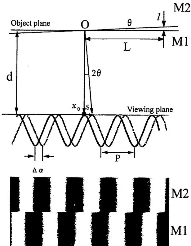
Fig. 1 Schematic of the rotation-angle measurement. M1, reference mirror; M2, object mirror; s, fringe shift;  $\Delta\alpha$ , phase difference;  $P$ , grating pitch;  $d$ , viewing distance.
