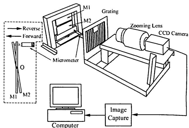
Fig. 3 Experimental setup:  $M1$ , reference mirror;  $M2$ , object mirror. Inset surrounded by dashed line shows how  $M2$  is rotated.
