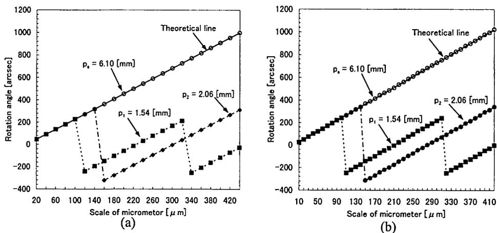
Fig. 10 Rotation angles measured in (a) the simulation and (b) the experiment. Plots on the dot-dash line and the dotted line are obtained by an ordinary method that uses a single grating. Plots on the solid line are obtained by a two-grating method.
