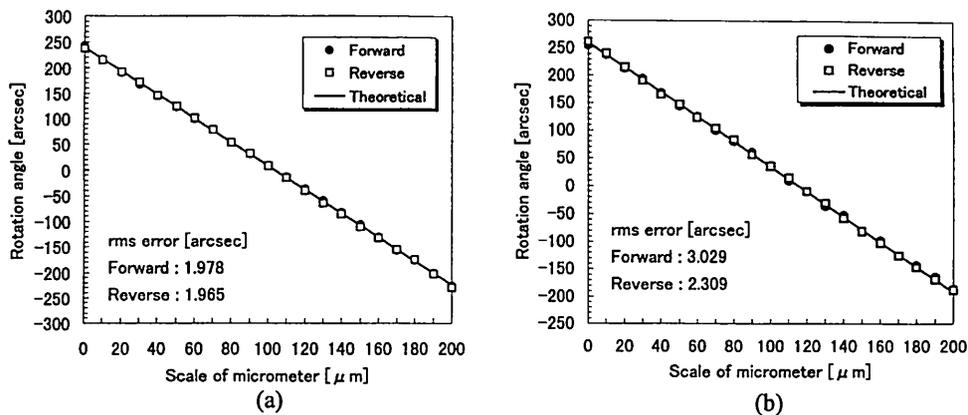
Fig. 9 Rotation angles measured with (a) the sinusoidal grating and (b) the binary grating. Travel pitches of the micrometer head are  $10 \mu\text{m}$ .
