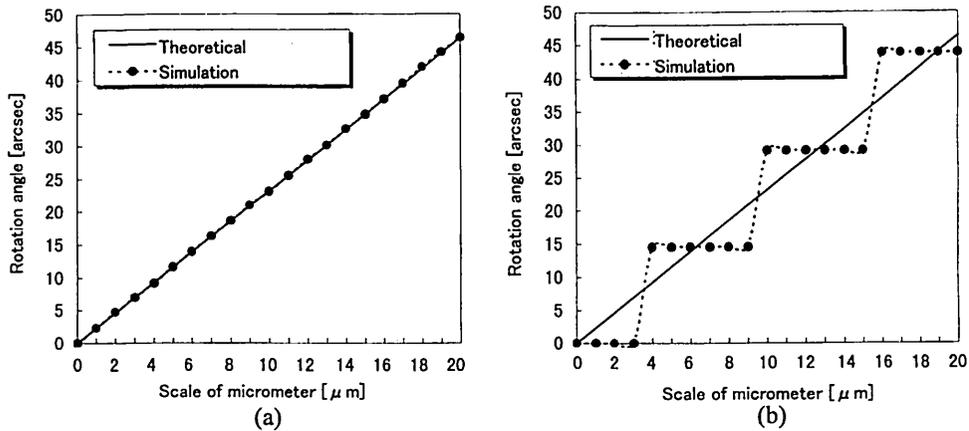
Fig. 7 Measurement error calculated by a simulation with (a) the sinusoidal grating and (b) the binary grating.
