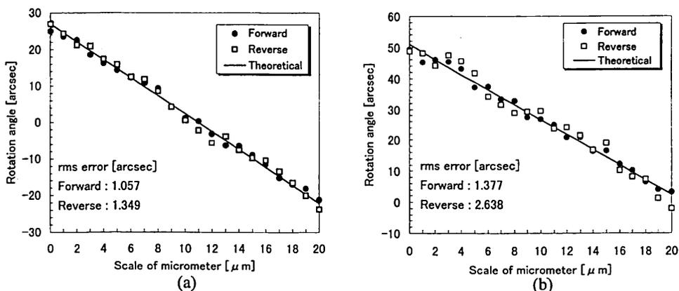
Fig. 8 Rotation angles measured with (a) the sinusoidal grating and (b) the binary grating. Travel pitches of the micrometer head are 1  $\mu\text{m}$ .
