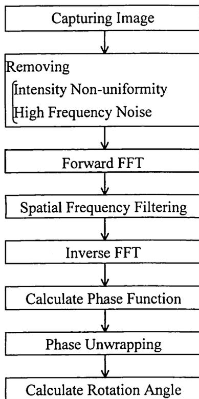
Fig. 2 Flow chart of the image processing.
