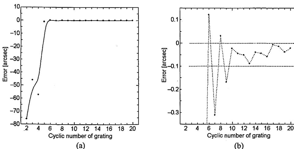
Fig. 6 Measurement error plotted against the cycle number of the grating: (a) overall plot and (b) magnification.
