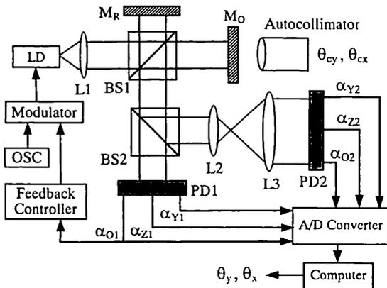
Fig. 4 Schematic of the experimental setup.
