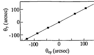
Fig. 8 Measured values of  $\theta_y$  obtained from phases  $\beta_{Z1}$  and  $\beta_{Z2}$  for rotation angle  $\theta_y$ .
