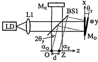
Fig. 1 Measurement of a 1-D rotation angle  $\theta_y$  with a Twyman-Green interferometer.
