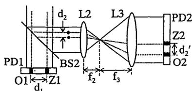
Fig. 2 Detection configuration to extend the measurement range.
