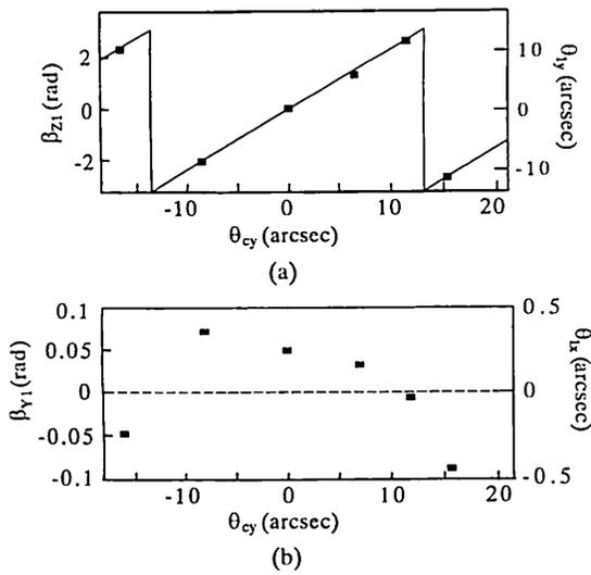
Fig. 6 Measured values of phases (a)  $\beta_{Z1}$  and (b)  $\beta_{Y1}$  for rotation angle  $\theta_y$ .
