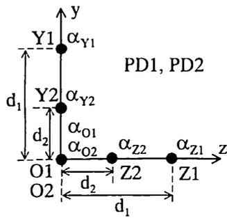
Fig. 3 Positions of the detection points and phases detected by PD1 and PD2.
