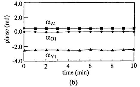
Fig. 5 Phase fluctuations (a) when the feedback control did not work and (b) when it worked for the phase  $\alpha_{O1}$  to be kept at 0 rad.
