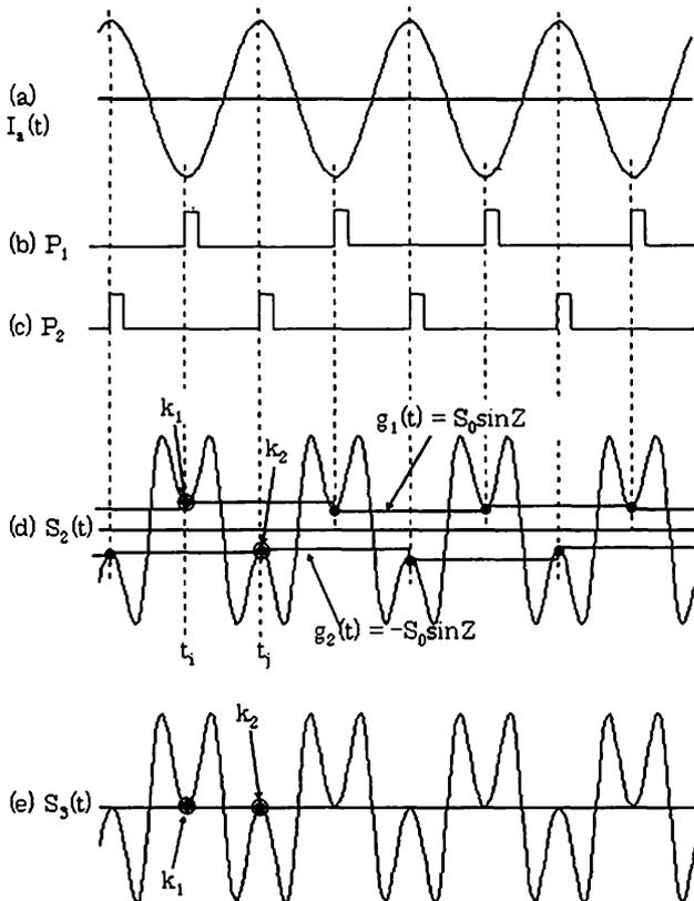
Fig. 4 Schematic of the feedback control: (a) sinusoidal signal for the phase modulation, (b) and (c) sampling pulses, (d) phase-locked signal and generation of the feedback signal, (e) phase-locked and modulation-amplitude-locked signal.
