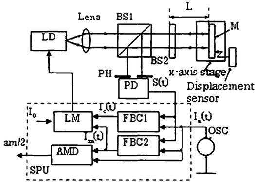
Fig. 1 Experimental setup: LD, laser diode; BS, beamsplitters; M, mirror; PH, pinhole; PD, photodiode; LM, laser modulator; FBC, feedback controllers; OSC, oscillator; AMD, amplitude detector.
