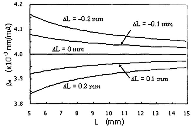
Fig. 6 Dependence of  $\beta$  on OPD error.
