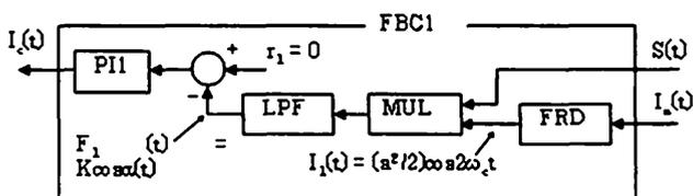
Fig. 2 Block diagram of FBC1: MUL, multiplier; LPF, lowpass filter; FRD, frequency doubler; PI1, proportional-integral controller.
