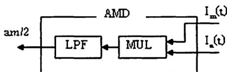
Fig. 5 Block diagram of the amplitude detector: MUL, multiplier; LPF, lowpass filter.
