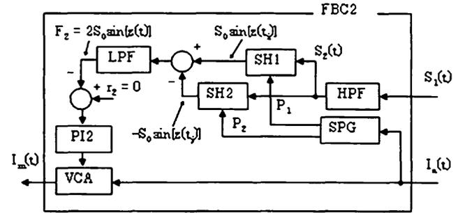
Fig. 3 Block diagram of FBC2: HPF, highpass filter; SPG, sampling pulse generator; SH, sample-and-hold circuits; LPF, lowpass filter; PI2, proportional-integral controller; VCA, voltage-controlled amplifier.
