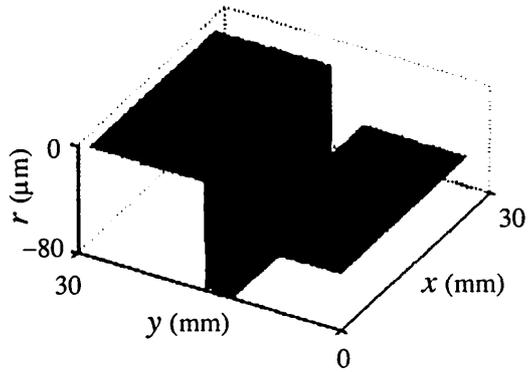
Fig. 10 Measured profile of the polished step surface in the  $x$ - $y$  plane.
