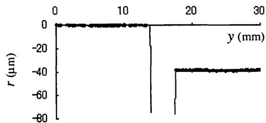
Fig. 11 Measured profile of the step surface on the line of  $x=15$  mm.
