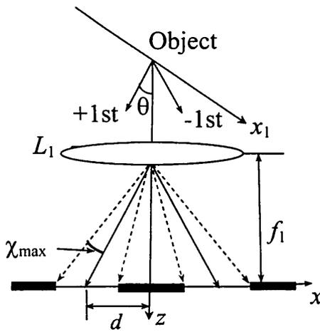
Fig. 3 Relations between the reflected lights and the slits on diaphragm  $H_1$ .
