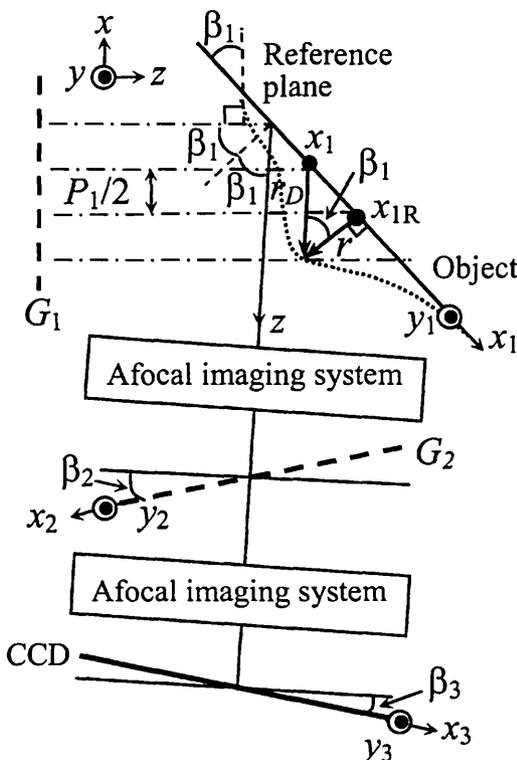
Fig. 2 Afocal imaging systems for the interference fringe pattern on an object.
