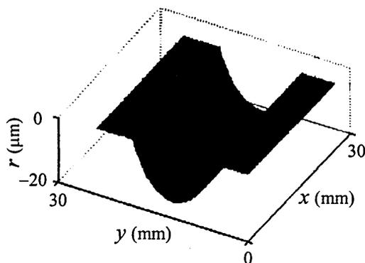
Fig. 5 Measured profile of the polished metal surface in the  $x$ - $y$  plane.
