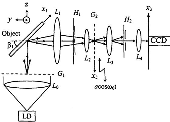
Fig. 1 Two-grating interferometer using sinusoidal phase-modulating interferometry.
