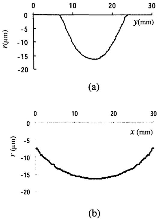
Fig. 8 Surface profile measured at the rotation angle  $\gamma$  of 10 deg on the two lines of (a)  $x=15$  mm and (b)  $y=15$  mm.
