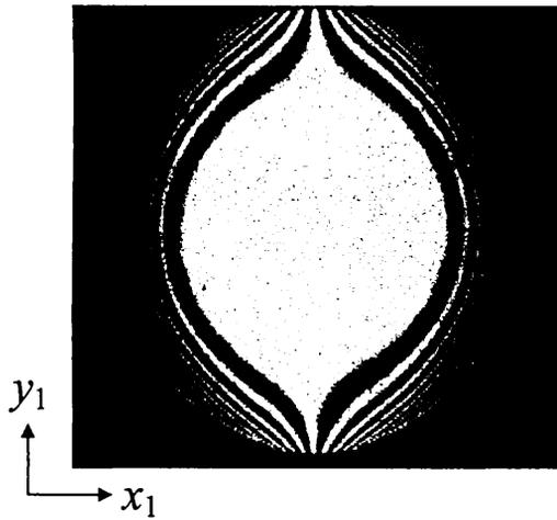
Fig. 4 Detected interference pattern involving the aberrations of a lens.
