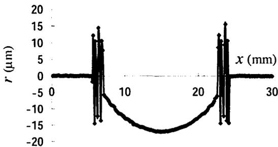
Fig. 9 Surface profile measured at the rotation angle  $\gamma$  of 12 deg on the line of  $y=15$  mm.
