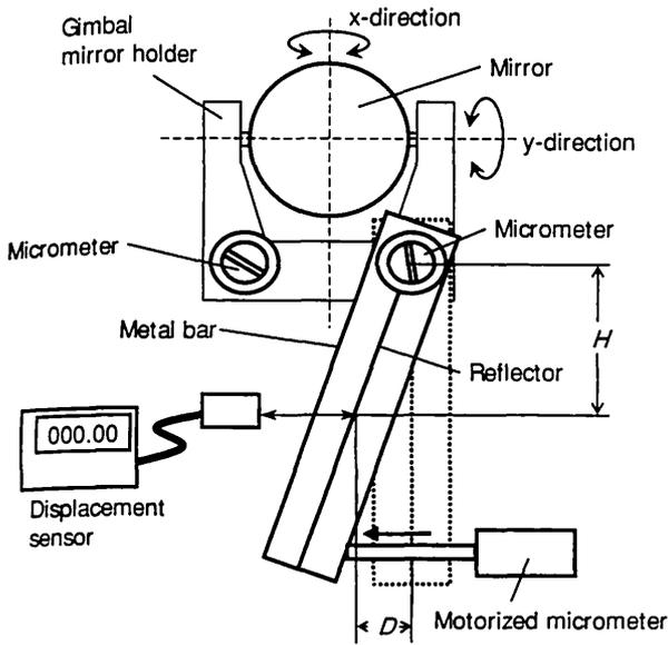
Fig. 5 Schematic of the mirror-rotating system.
