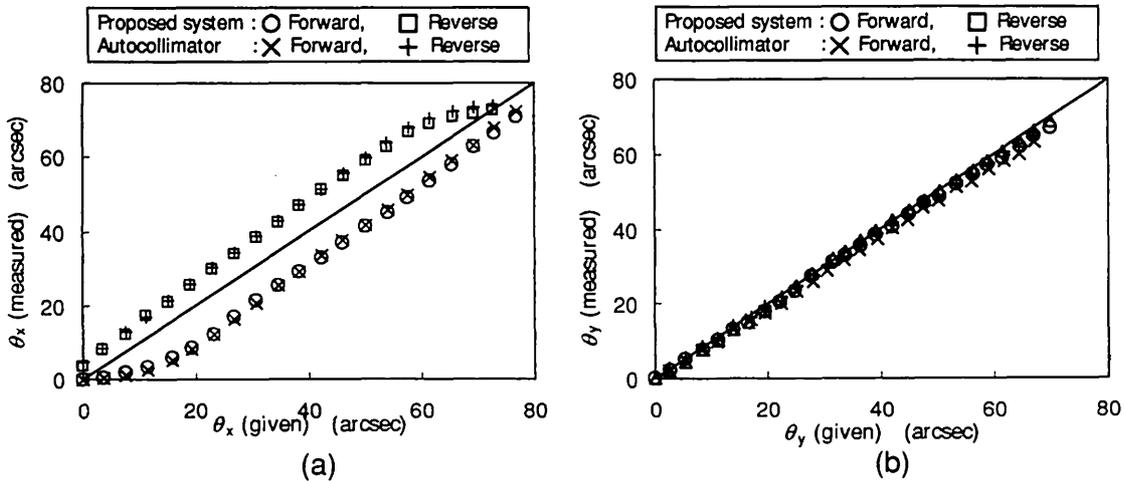
Fig. 6 Measured rotation angle for (a) the x direction and (b) the y direction in the range of 0 to 80 arcsec. "Forward" and "Reverse" mean increment and decrement of the angular displacement.
