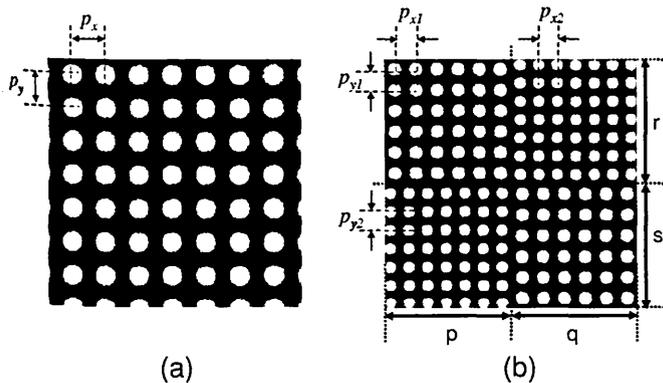
Fig. 2 Grating images (a) \$S1\$ of the 1-D grating and (b) \$S2\$ of the 2-D grating used in the experiments. \$S2\$ is divided into four sections.
