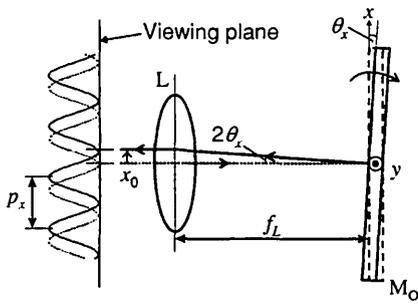
Fig. 1 Principle of the measurement: \$M\_O\$, object mirror; \$L\$, imaging lens; \$x\_0\$, fringe shift; \$p\_x\$, pitch of the grating; \$f\_L\$, focal length of the imaging lens.
