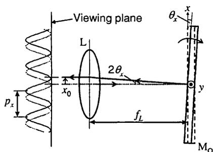
Fig. 1 Principle of the measurement:  $M_0$ , object mirror; L, imaging lens;  $x_0$ , fringe shift;  $p_x$ , pitch of the grating;  $f_L$ , focal length of the imaging lens.
