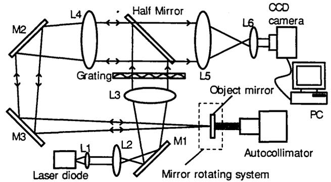
Fig. 4 Experimental setup: L, lenses; M, mirrors; PC, computer.
