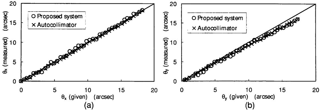
Fig. 7 Measured rotation angle for (a) the x direction and (b) the y direction in the range of 0 to 20 arcsec. The measurement was made in the "Forward" direction.
