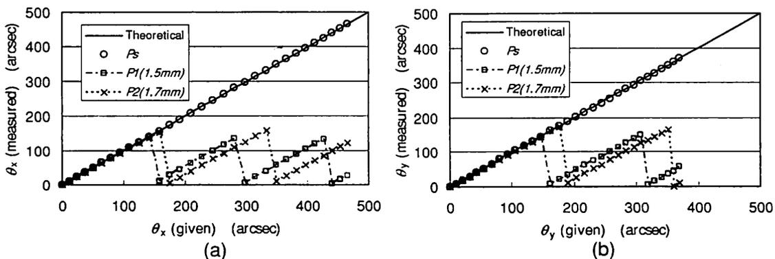
Fig. 8 Rotation angles for (a) the x direction and (b) the y direction measured with two-pitch grating S2. Plots on the dot-dash line and dotted line are obtained with a single pitch. Plots on the solid line are obtained by the two-pitch method.
