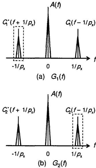
Fig. 3 Distribution of the Fourier spectra of (a)  $G_1(f)$  and (b)  $G_2(f)$ . The phase difference is calculated by using the components enclosed in the dashed rectangles.
